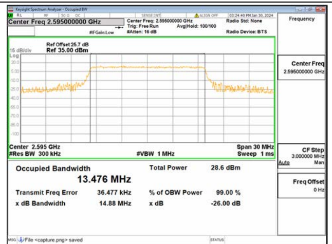
B38 / 15MHz / 64QAM/ Mid CH
