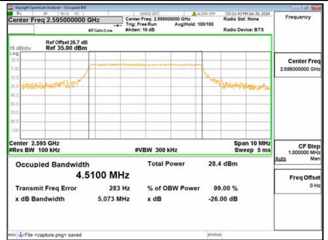
B38 / 5MHz / 64QAM/ Mid CH
