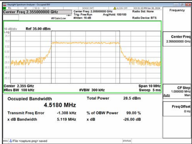
B40-2 / 5MHz / 16QAM / Mid CH
