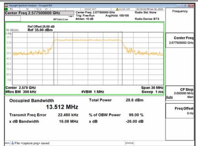
B38 / 15MHz / 16QAM/ Low CH
