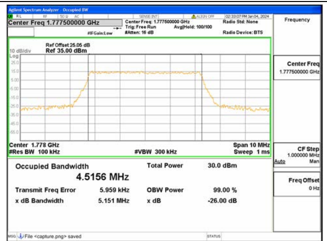
B66 / 5MHz / 16QAM/ High CH
