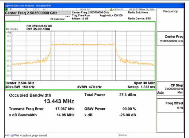
B41 / 15MHz / 16QAM/ Low CH
