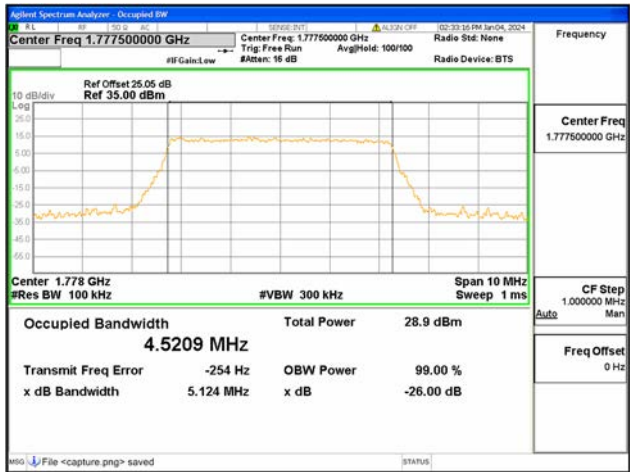
B66 / 5MHz / 64QAM/ High CH
