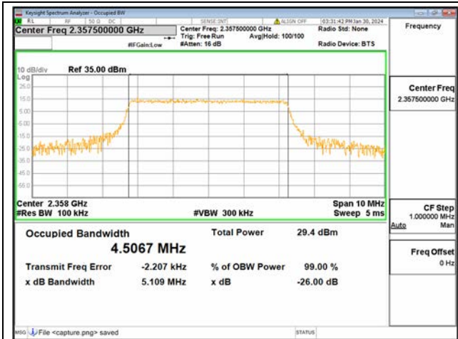
B40-2 / 5MHz / QPSK/ High CH
