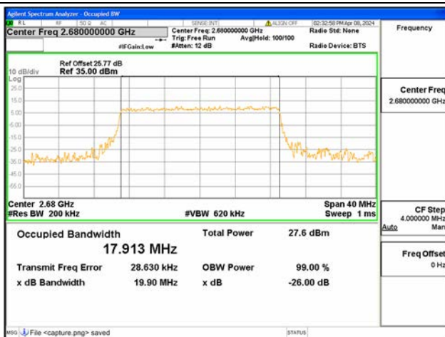
B41 / 20MHz / 16QAM / High CH
