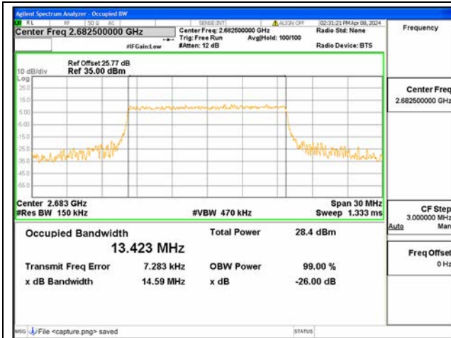
B41 / 15MHz / QPSK/ High CH
