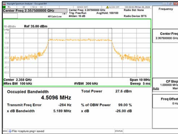
B40-2 / 5MHz / 64QAM/ High CH
