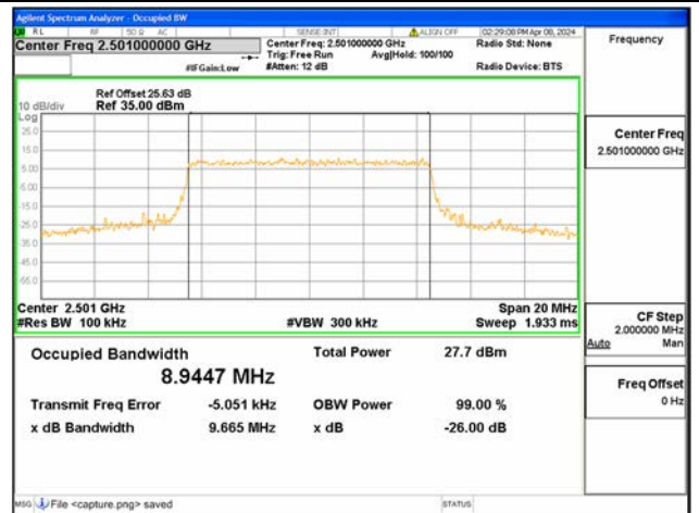
B41 / 10MHz / 64QAM/ Low CH
