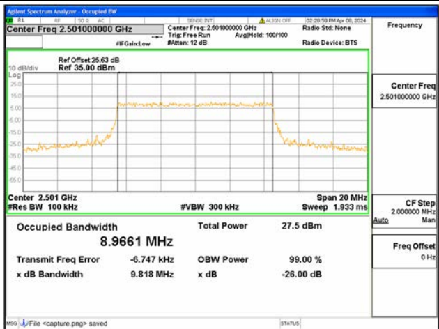
B41 / 10MHz / 16QAM/ Low CH
