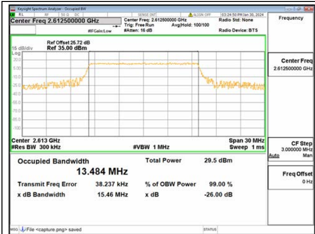
B38 / 15MHz / QPSK/ High CH
