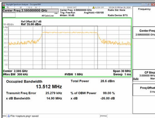
B38 / 15MHz / 16QAM/ Mid CH
