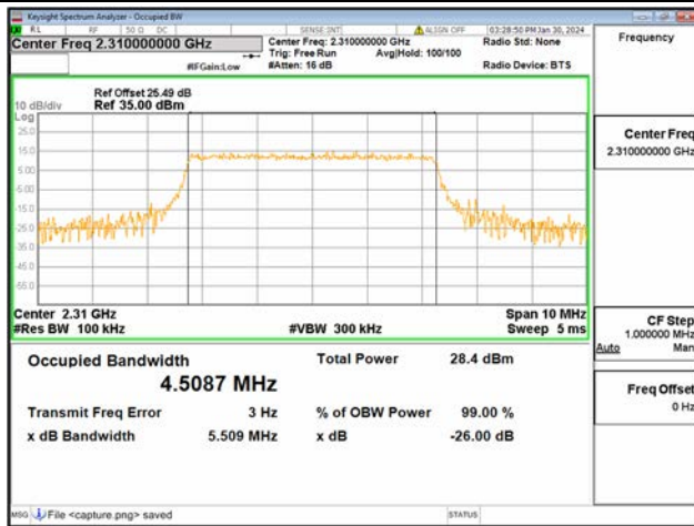
B40-1 / 5MHz / 16QAM / Mid CH
