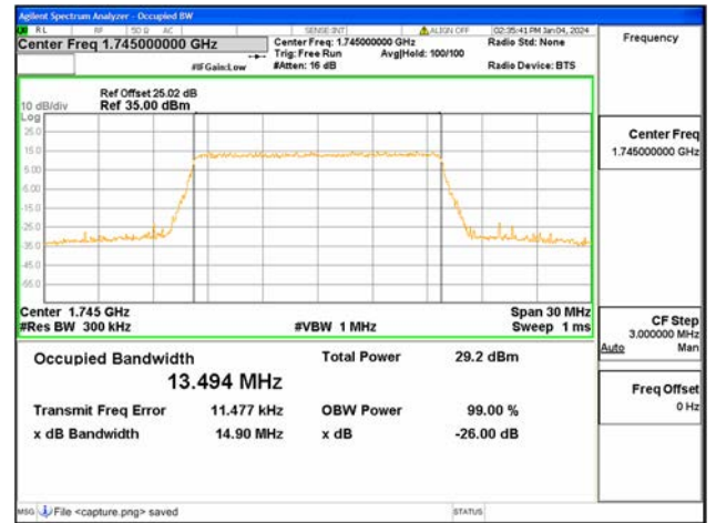
B66 / 15MHz / 64QAM/ Mid CH
