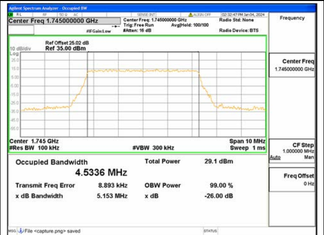
B66 / 5MHz / 64QAM/ Mid CH
