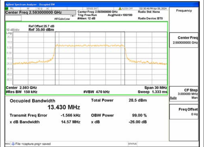
B41 / 15MHz / QPSK/ Mid CH
