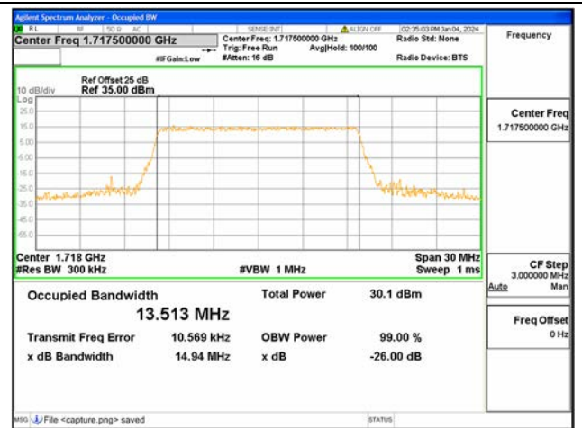
B66 / 15MHz / 16QAM/ Low CH
