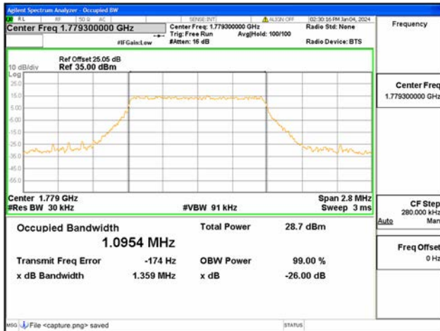
B66 / 1.4MHz / 64QAM/ High CH
