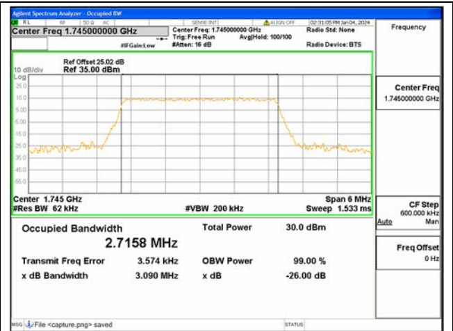
B66 / 3MHz / 16QAM/ Mid CH
