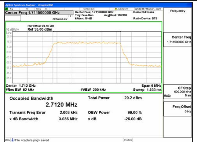
B66 / 3MHz / 64QAM/ Low CH
