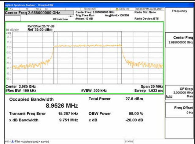
B41 / 10MHz / 64QAM / High CH
