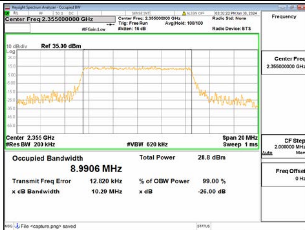
B40-2 / 10MHz / 16QAM/ Mid CH
