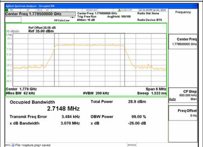
B66 / 3MHz / 64QAM/ High CH
