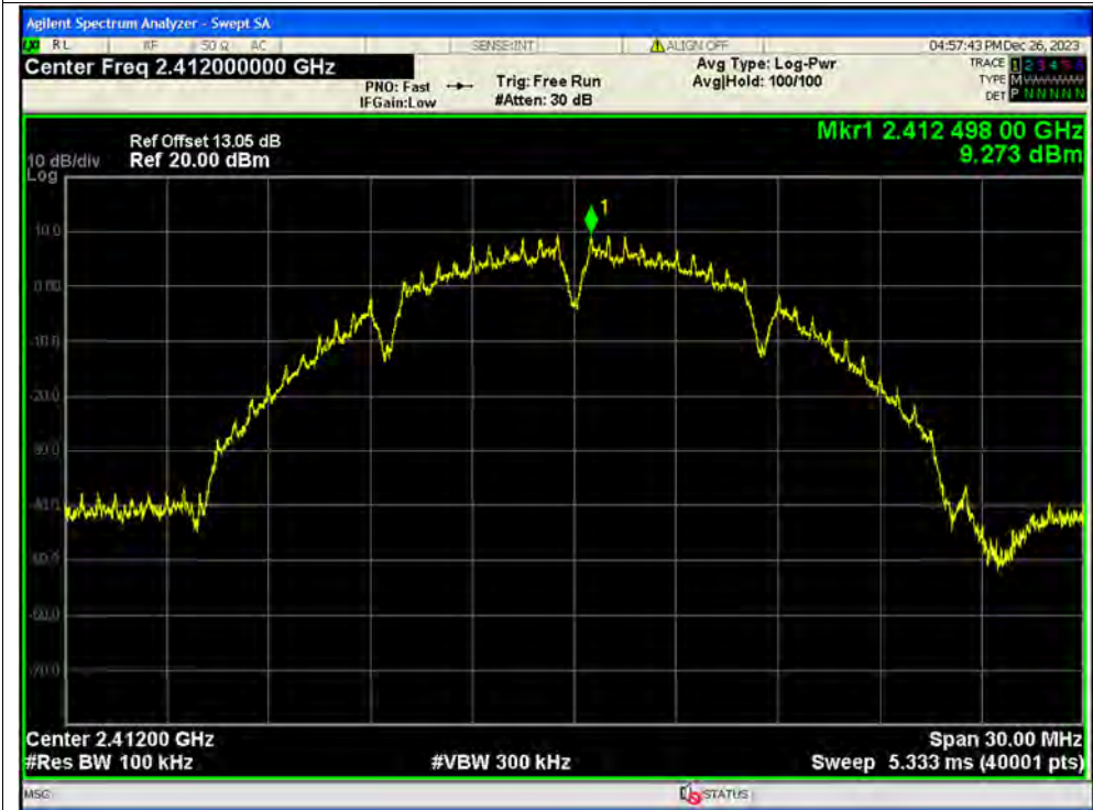
Tx. Spurious NVNT b 2412MHz Ant1 Emission
