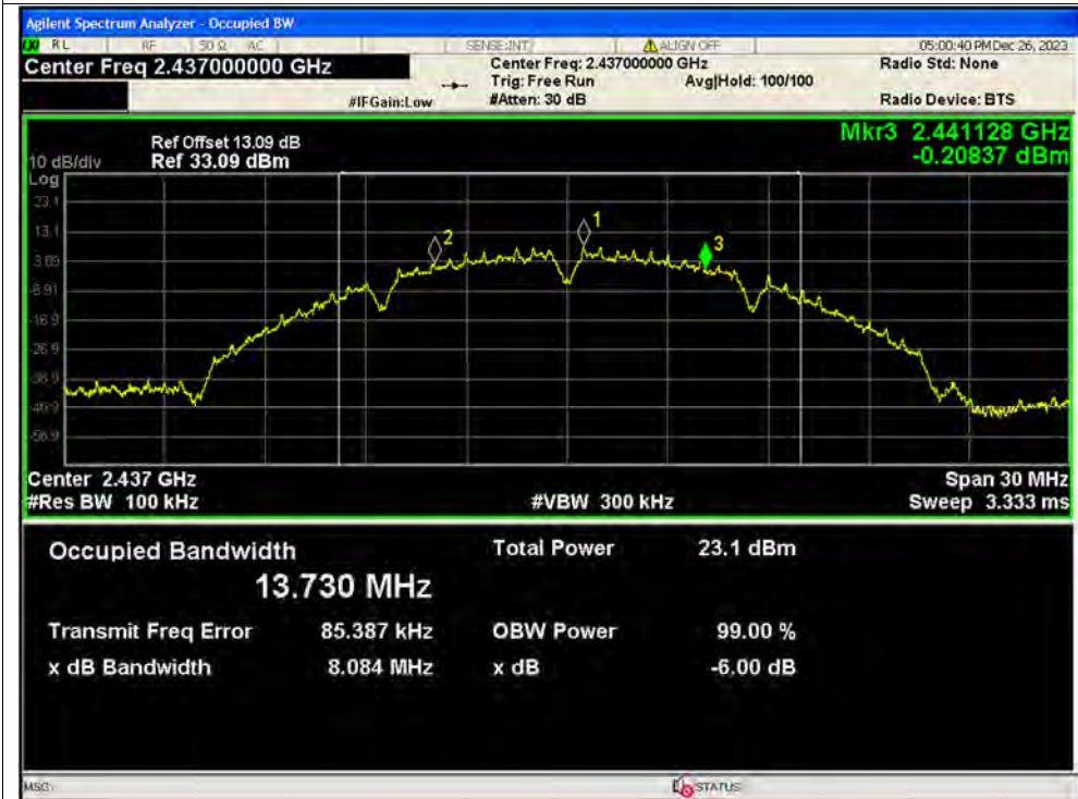
-6dB Bandwidth NVNT b 2437MHz Ant1
