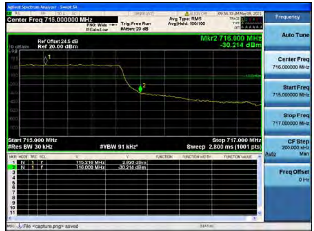
Band12 / 1.4MHz / High CH / QPSK / FULL RB
