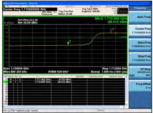
Band4 / 20MHz / High CH / QPSK / FULL RB
