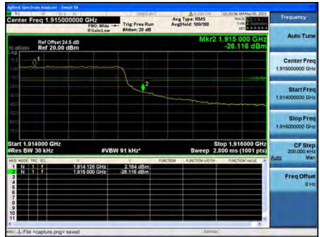
Band25 / 1.4MHz / High CH / QPSK / FULL RB
