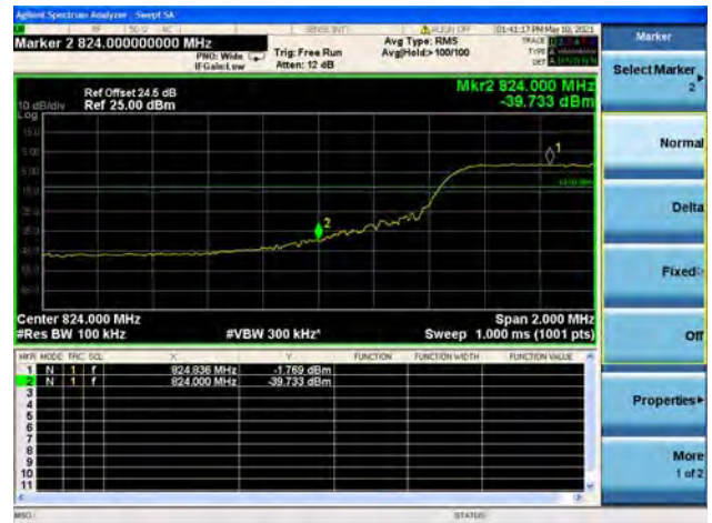
Band26 / 10MHz / High CH / QPSK / FULL RB
