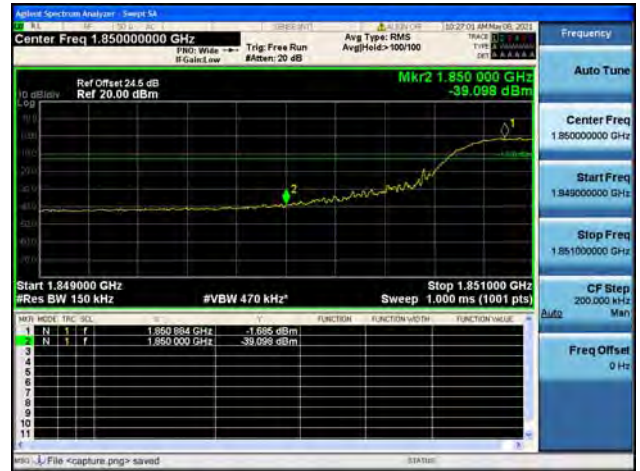
Band25 / 15MHz / High CH / QPSK / FULL RB
