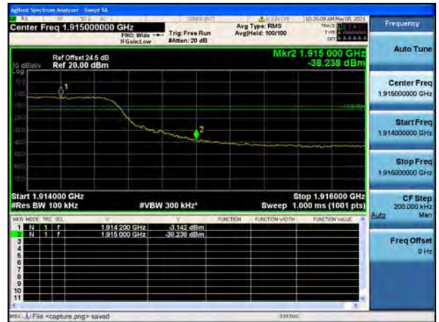
Band25 / 10MHz / High CH / QPSK / FULL RB
