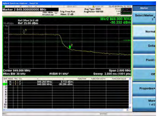
Band26 / 1.4MHz / High CH / QPSK / FULL RB
