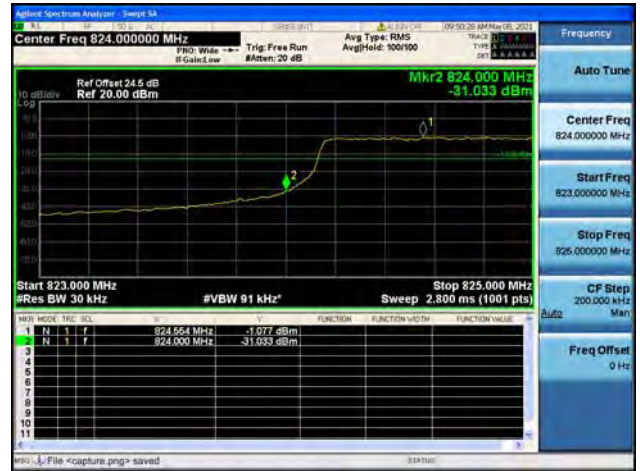
Band5 / 3MHz / High CH / QPSK / FULL RB
