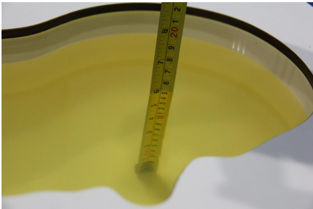
Picture 7-1: Liquid depth in the Head Phantom(3500MHz)
