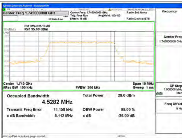
B66 / 5MHz / 64QAM/ Mid CH
