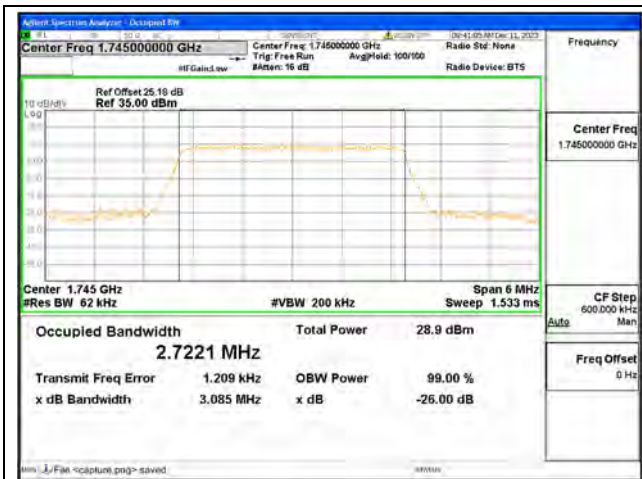
B66 / 3MHz / 64QAM/ Mid CH
