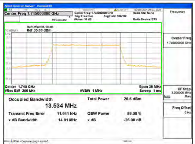
B66 / 15MHz / 256QAM/ Mid CH
