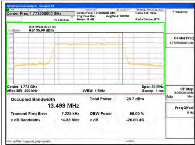
B66 / 15MHz / 64QAM/ High CH
