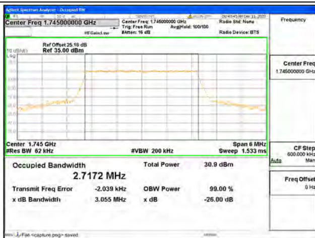
B66 / 3MHz / QPSK/ Mid CH
