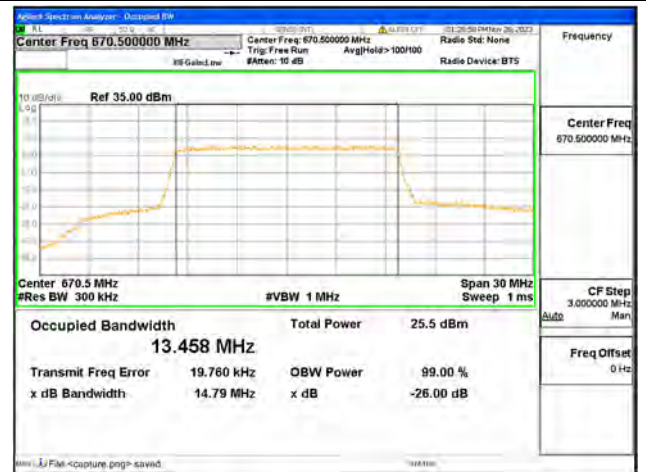
B71 / 15MHz / 256QAM/ Low CH
