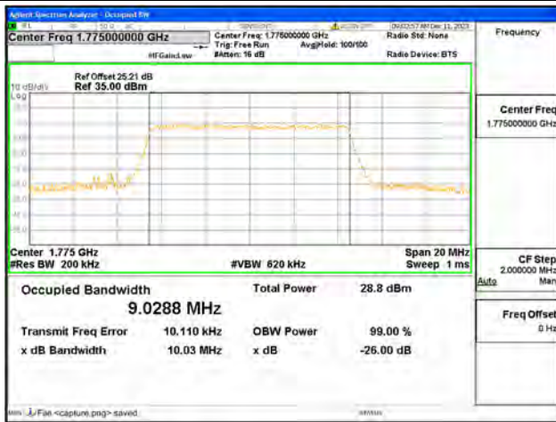
B66 / 10MHz / 64QAM/ High CH
