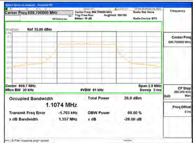
B12 / 1.4MHz / 256QAM/ Low CH
