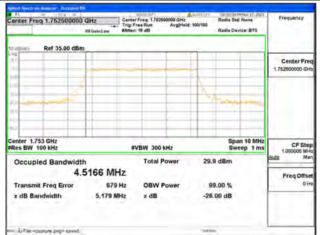
B4 / 5MHz / 16QAM/ High CH
