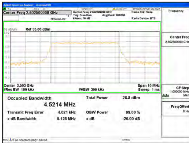
B7 / 5MHz / 64QAM/ Low CH
