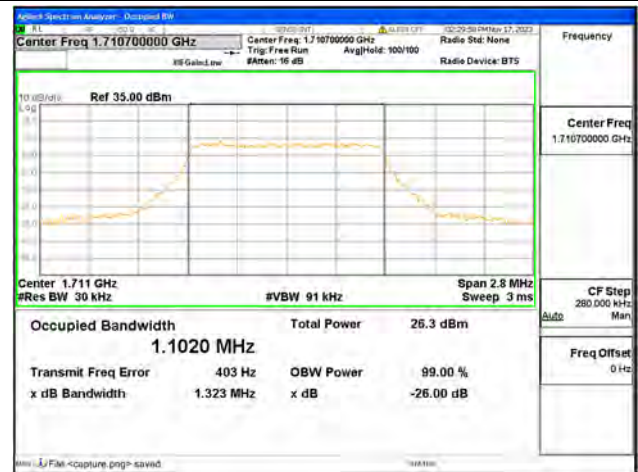
B4 / 1.4MHz / 256QAM/ Low CH
