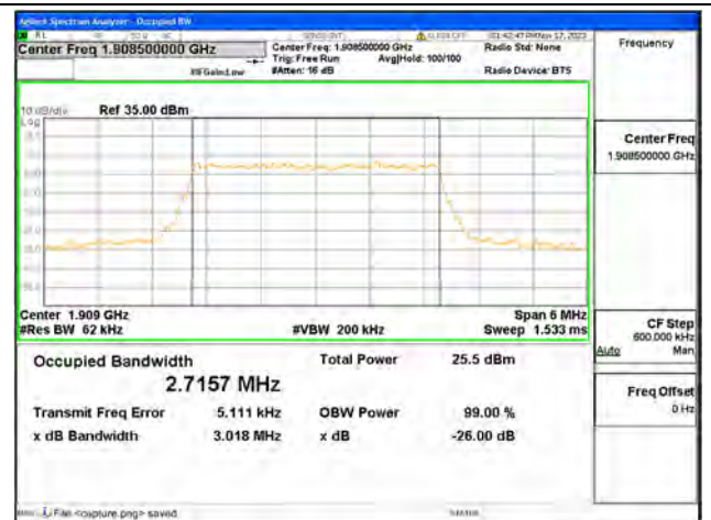
B2 / 3MHz / 256QAM/ High CH
