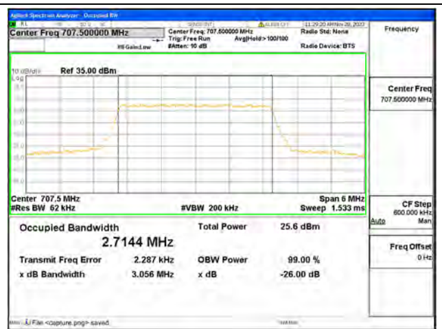
B12 / 3MHz / 256QAM/ Mid CH
