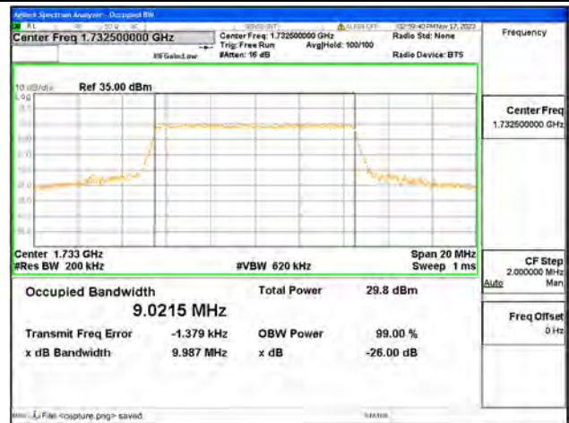
B4 / 10MHz / 16QAM/ Mid CH
