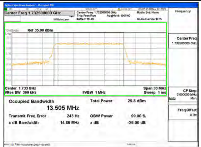
B4 / 15MHz / 16QAM/ Mid CH
