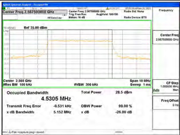
B7 / 5MHz / 64QAM/ High CH
