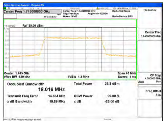
B4 / 20MHz / 256QAM/ High CH
