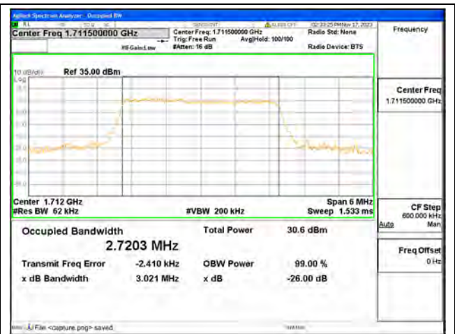
B4 / 3MHz / 16QAM/ Low CH
