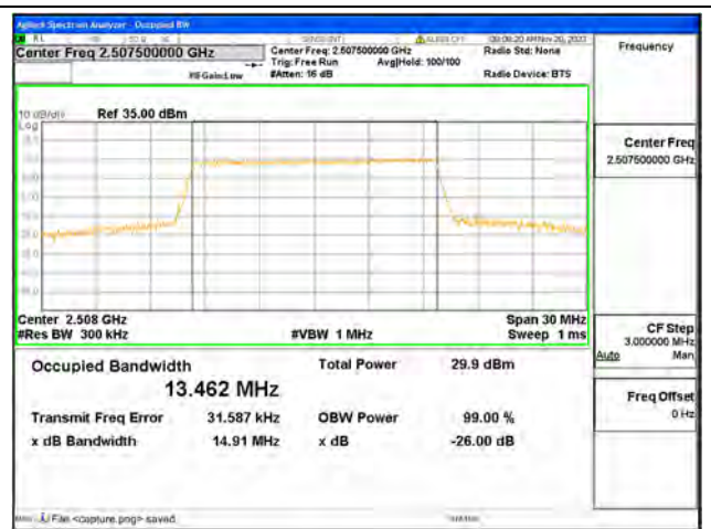
B7 / 15MHz / 16QAM/ Low CH
