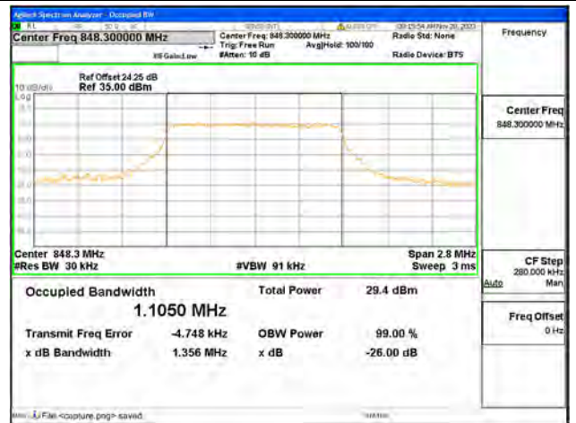
B5 / 1.4MHz / 16QAM/ High CH
