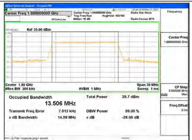
B2 / 15MHz / 16QAM/ Mid CH
