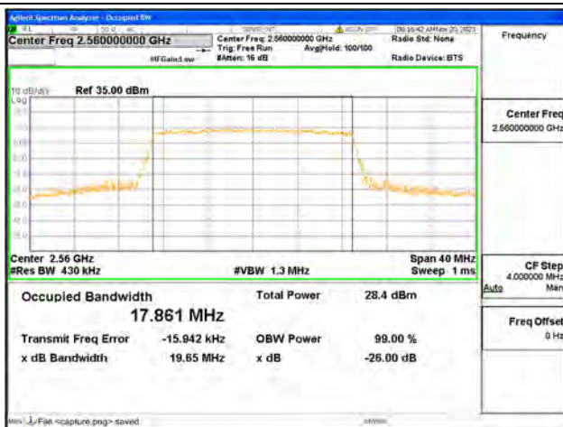
B7 / 20MHz / 64QAM/ High CH
