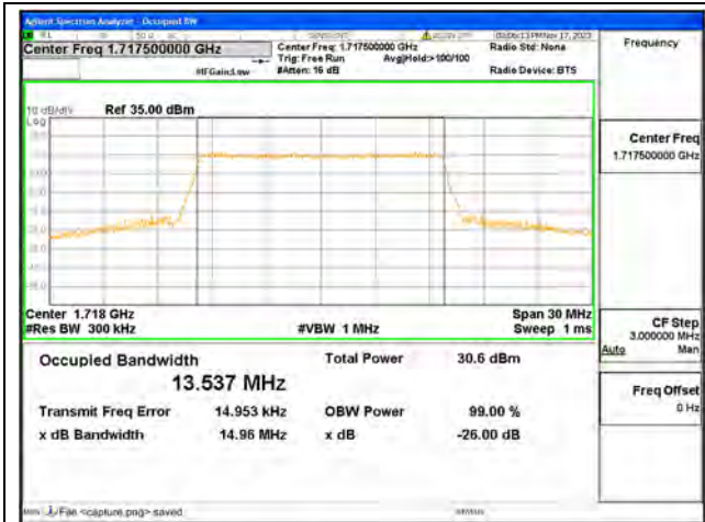
B4 / 15MHz / QPSK/ Low CH
