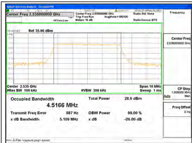
B7 / 5MHz / 64QAM/ Mid CH
