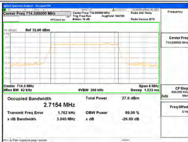
B12 / 3MHz / 64QAM/ High CH
