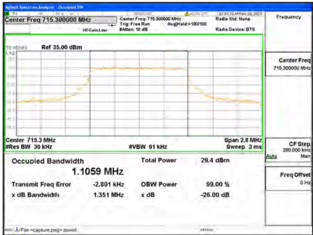
B12 / 1.4MHz / QPSK/ High CH
