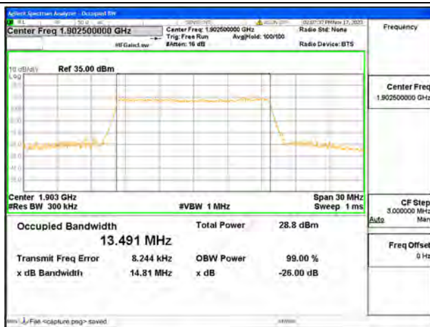
B2 / 15MHz / 64QAM/ High CH
