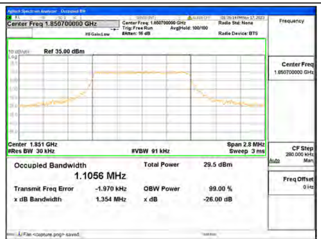
B2 / 1.4MHz / 16QAM/ Low CH
