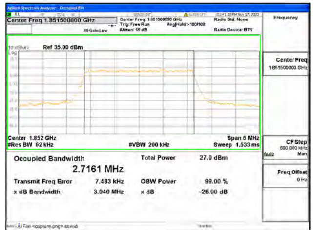
B2 / 3MHz / 256QAM / Low CH
