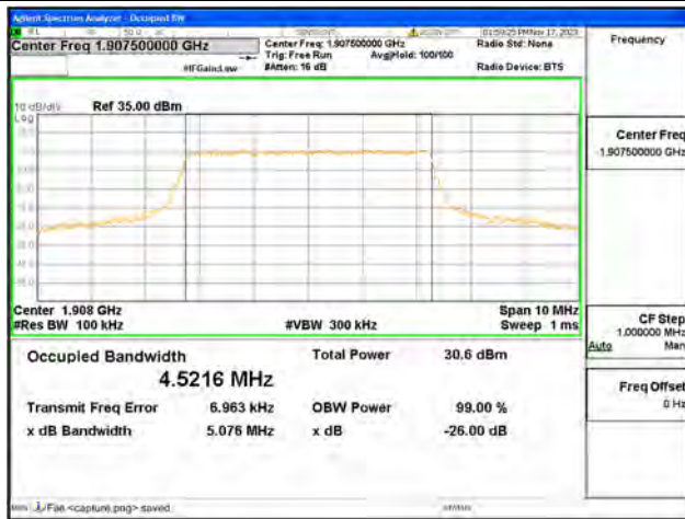
B2 / 5MHz / QPSK/ High CH
