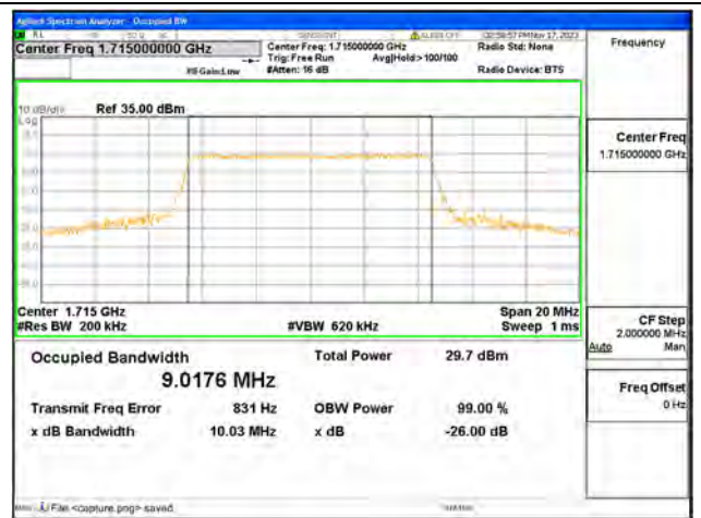
B4 / 10MHz / 16QAM/ Low CH
