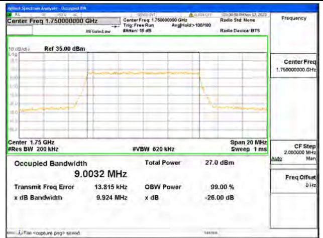
B4 / 10MHz / 256QAM/ High CH
