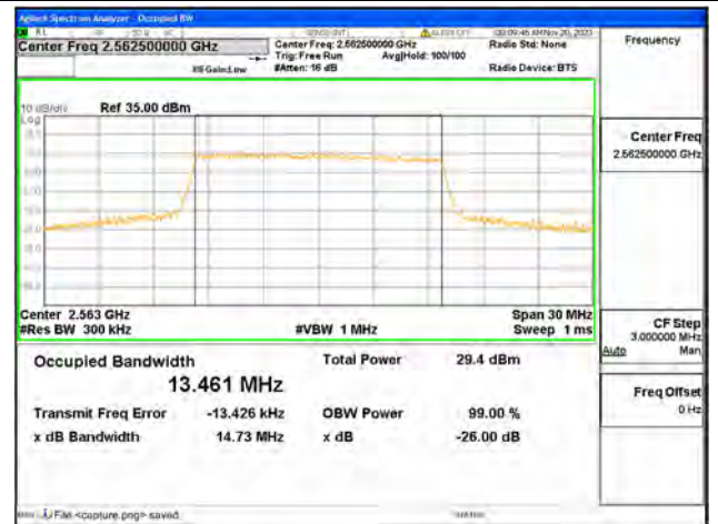
B7 / 15MHz / 16QAM/ High CH
