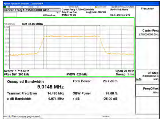
B4 / 10MHz / 256QAM/ Low CH
