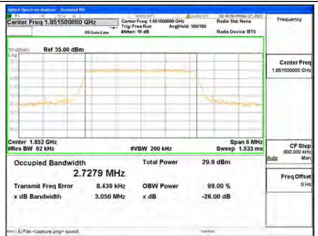
B2 / 3MHz / 16QAM / Low CH
