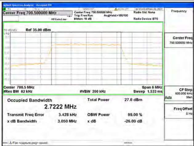
B12 / 3MHz / 64QAM/ Low CH
