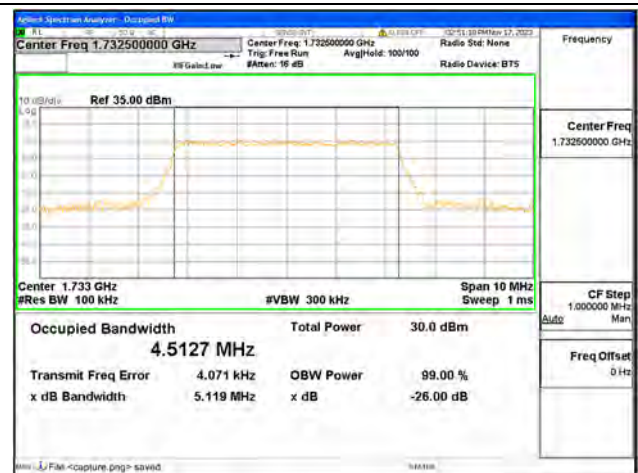
B4 / 5MHz / 16QAM / Mid CH
