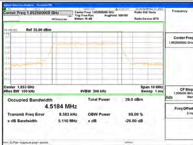
B2 / 5MHz / 64QAM/ Low CH
