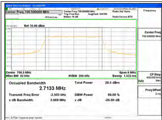
B12 / 3MHz / QPSK/ Low CH
