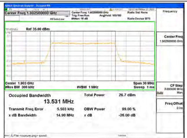
B2 / 15MHz / 256QAM/ High CH
