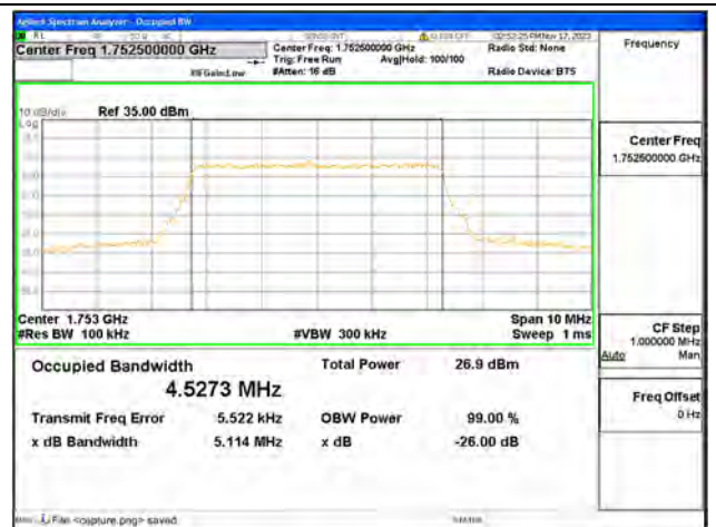
B4 / 5MHz / 256QAM/ High CH
