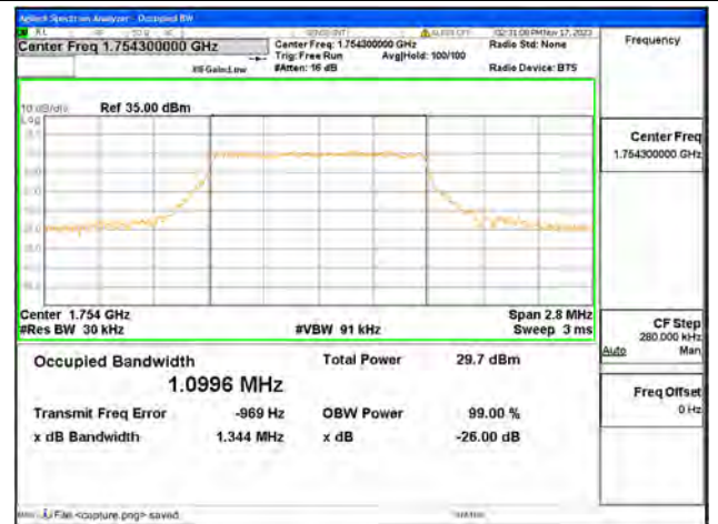
B4 / 1.4MHz / 16QAM/ High CH
