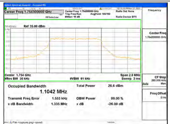
B4 / 1.4MHz / 256QAM/ High CH
