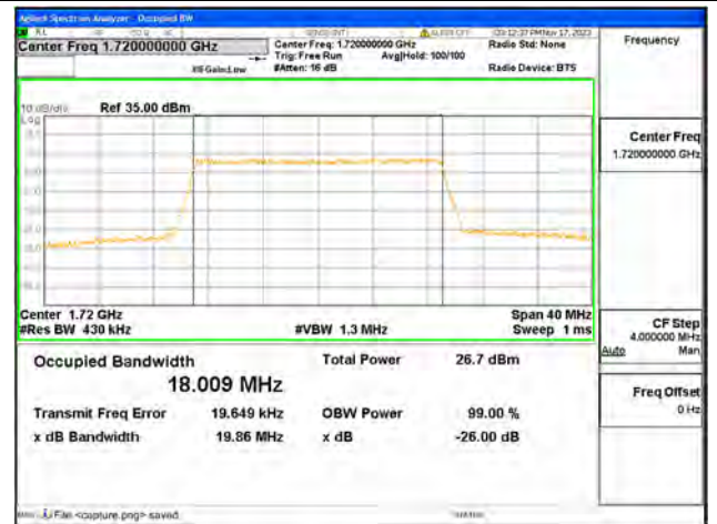
B4 / 20MHz / 256QAM/ Low CH
