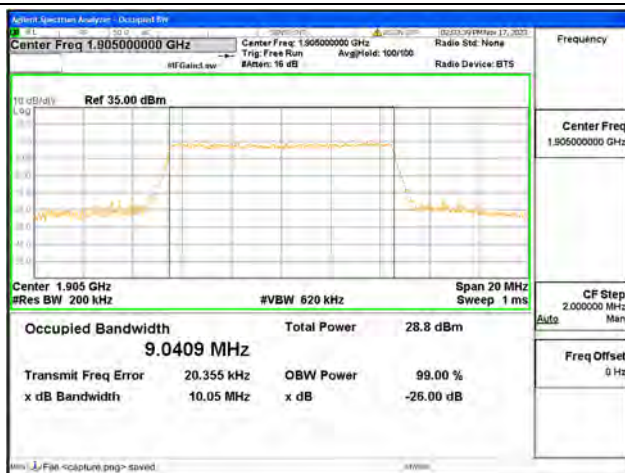
B2 / 10MHz / 64QAM/ High CH
