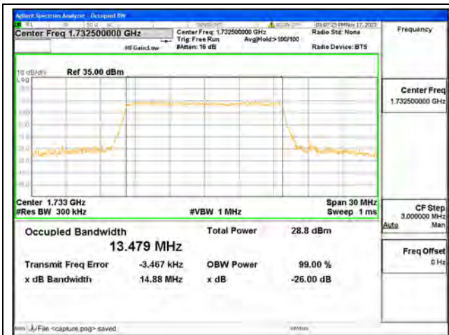
B4 / 15MHz / 64QAM/ Mid CH
