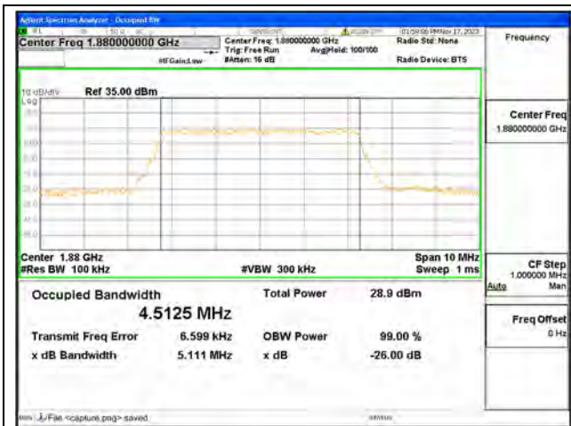
B2 / 5MHz / 64QAM/ Mid CH
