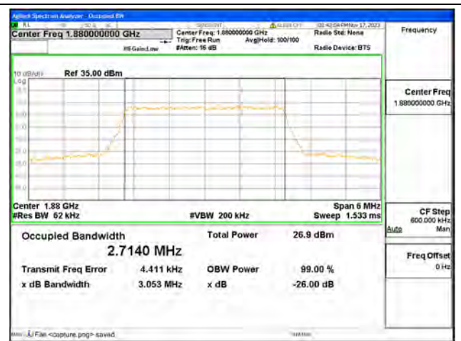
B2 / 3MHz / 256QAM/ Mid CH
