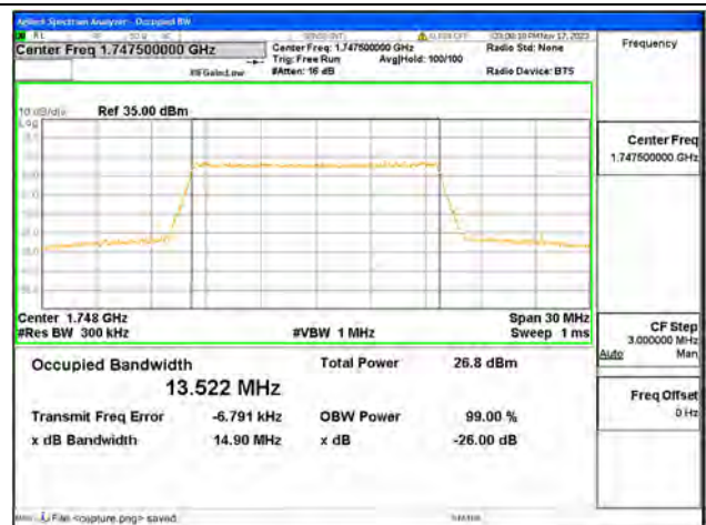
B4 / 15MHz / 256QAM/ High CH
