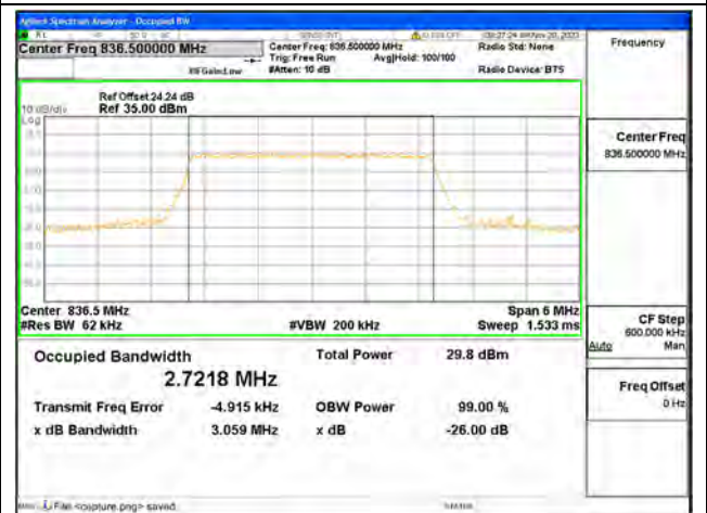
B5 / 3MHz / 16QAM/ Mid CH
