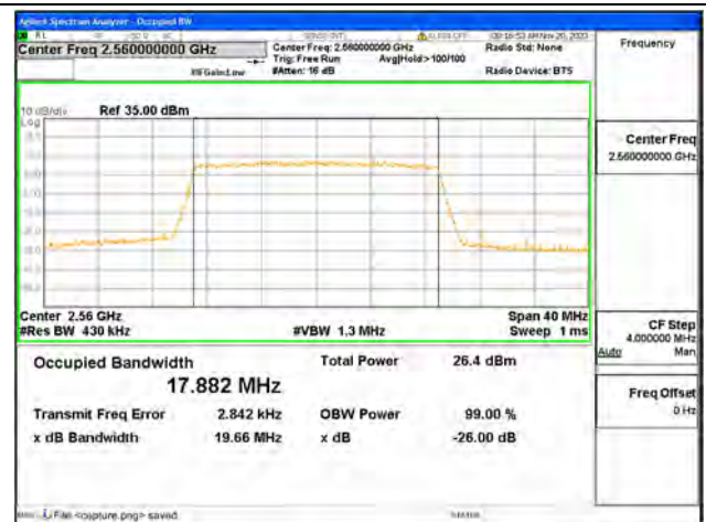
B7 / 20MHz / 256QAM/ High CH
