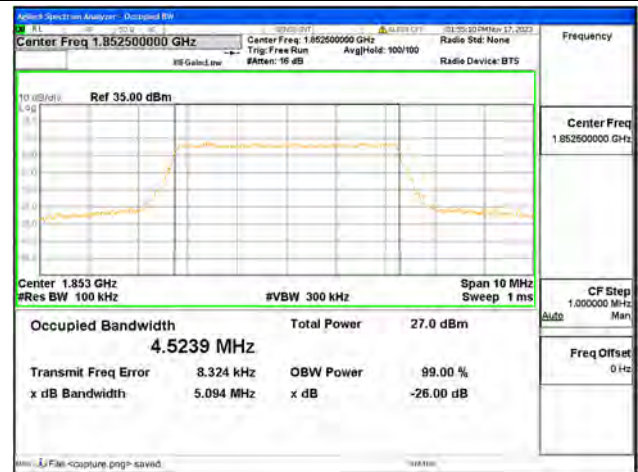
B2 / 5MHz / 256QAM/ Low CH
