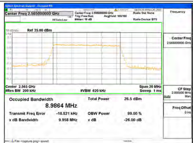
B7 / 10MHz / 256QAM/ High CH
