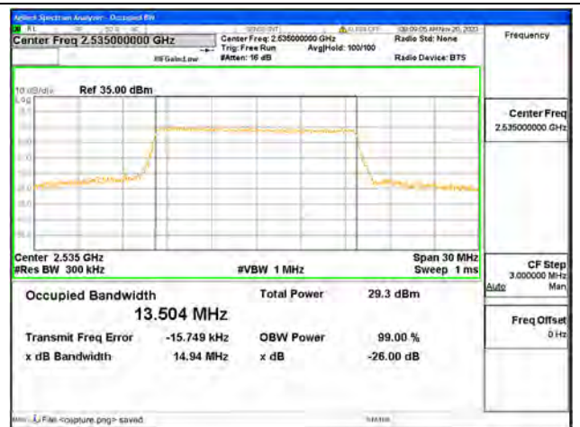
B7 / 15MHz / 16QAM/ Mid CH
