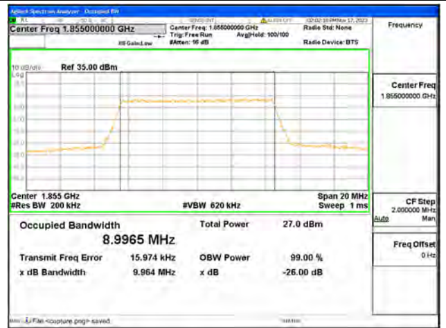
B2 / 10MHz / 256QAM/ Low CH
