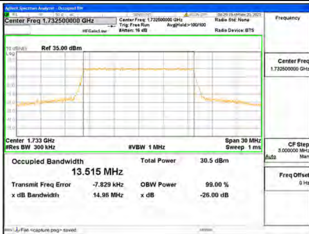
B4 / 15MHz / QPSK/ Mid CH
