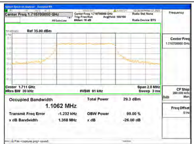
B4 / 1.4MHz / 16QAM/ Low CH
