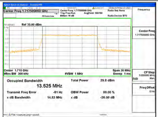
B4 / 15MHz / 16QAM/ Low CH
