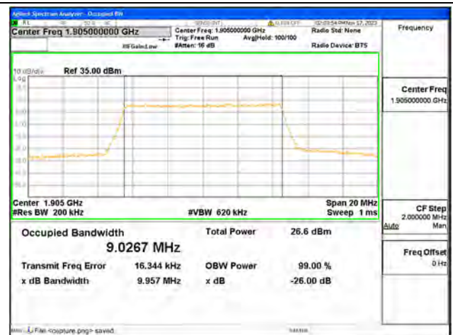
B2 / 10MHz / 256QAM/ High CH
