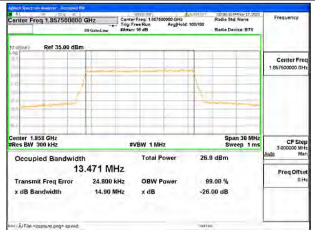
B2 / 15MHz / 256QAM/ Low CH
