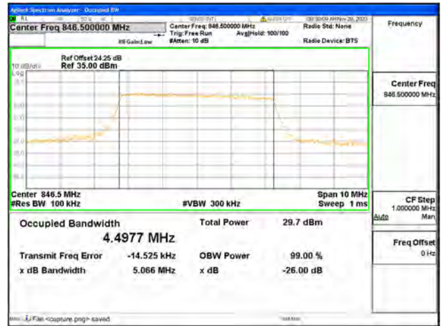
B5 / 5MHz / 16QAM/ High CH
