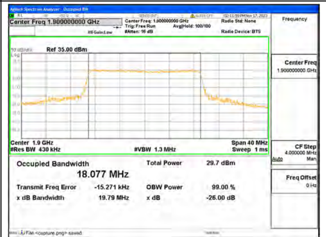
B2 / 20MHz / 16QAM/ High CH
