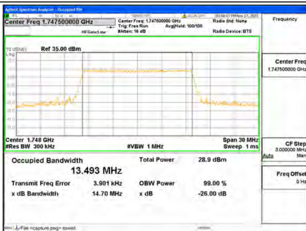
B4 / 15MHz / 64QAM/ High CH
