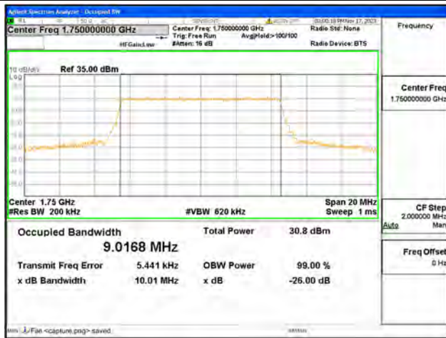
B4 / 10MHz / QPSK/ High CH
