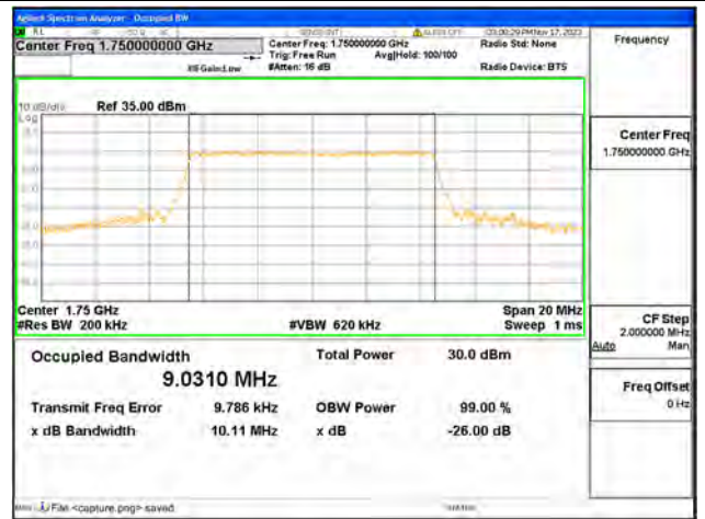
B4 / 10MHz / 16QAM/ High CH
