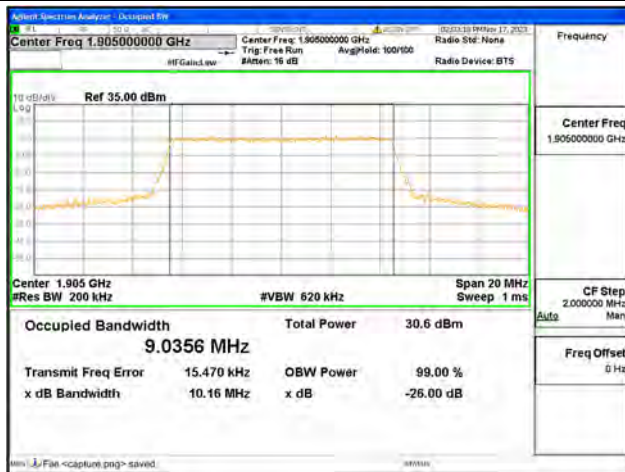
B2 / 10MHz / QPSK/ High CH
