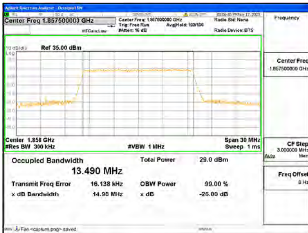
B2 / 15MHz / 64QAM/ Low CH
