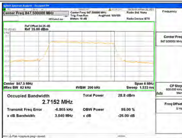
B5 / 3MHz / 64QAM/ High CH
