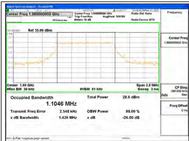
B2 / 1.4MHz / 64QAM/ Mid CH
