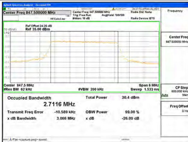
B5 / 3MHz / QPSK/ High CH
