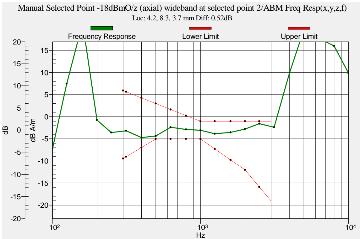
Figure 14: Frequency Response CDMA Cell – Channel 384
