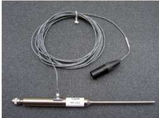
Figure 4: AM1D Probe with probe cable
