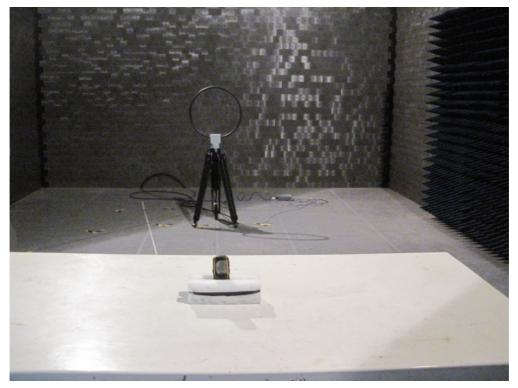
Test Mode : Mode 1: Transmit Description : Radiated Emission Test Setup for Below 1GHz
