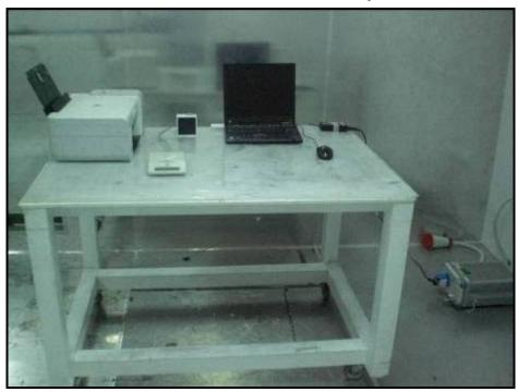
Radiated Emissions, 30 MHz to 1 GHz Test Setup
