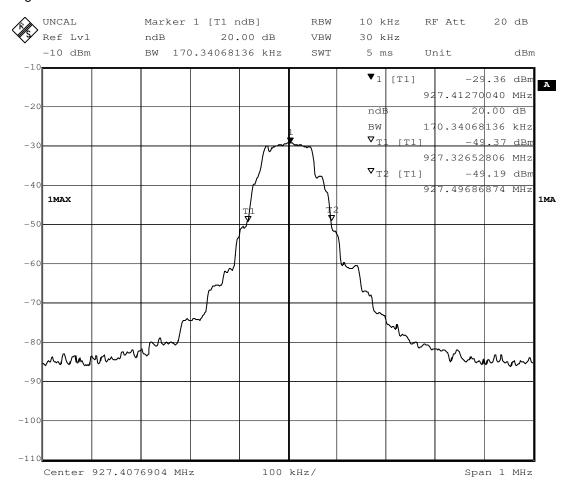
The low frequency is 927.32652806MHz, The high frequency is 927.49686874MHz, Within the band 902MHz to 928MHz.
