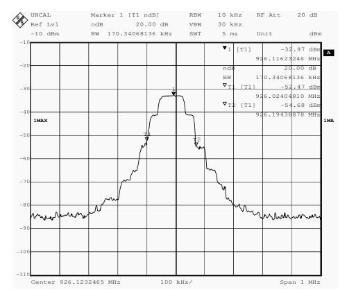
The low frequency is 926.02404810MHz, The high frequency is 926.19438878MHz, Within the band 902MHz to 928MHz.
