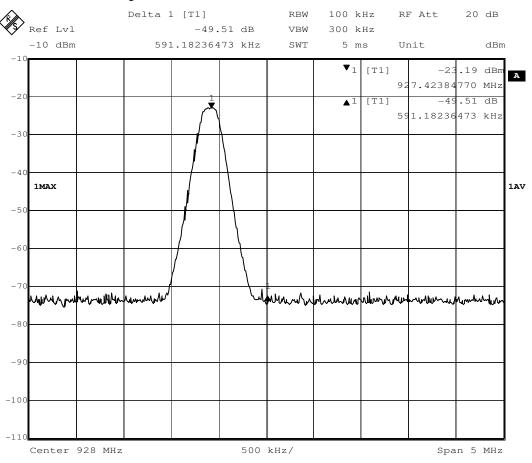
For 928MHz band edge checked with 927.4MHz frequency operated, the delta shown at the plots are -45.22dB for peak detector mode and -49.51dB for Average detector mode.
