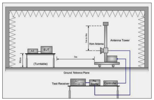
The field strength is calculated by adding the Antenna Factor, Cable Factor & Peramplifier . The basic equation with a sample calculation is as follows:
