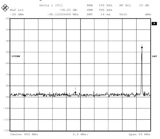
For 902MHz bandedge checked with 926.1MHz frequency operated, the delta shown at the plots are -35.19dB for peak detector mode and -38.23dB for Average detector mode.
