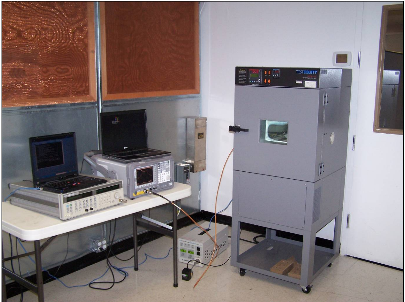
Photograph 11. Frequency Stability, Test Setup, M5 Radio
