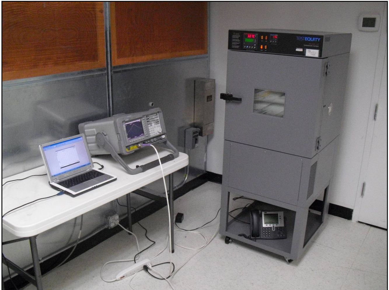
Photograph 6. Frequency Stability, Test Setup, M25 Radio
