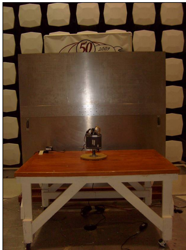
Photograph 3. Conducted Emissions, Test Setup, M25 Radio
