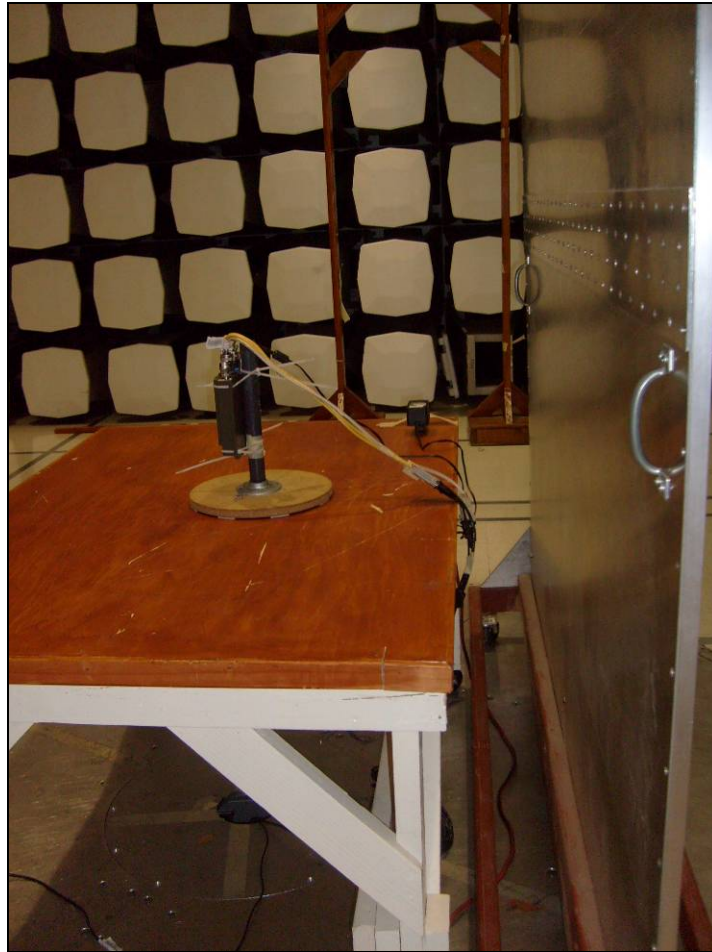
Photograph 4. Conducted Emissions, Test Setup, Side View, M25 Radio
