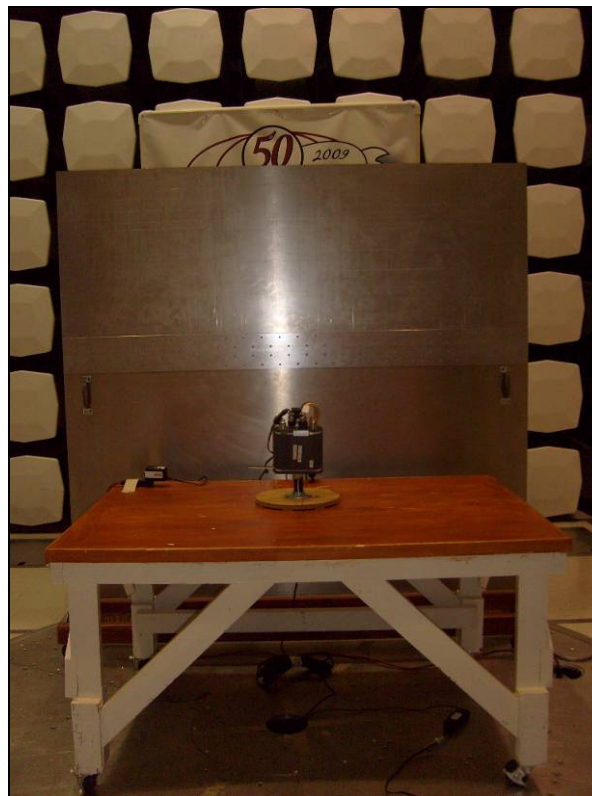
Photograph 8. Conducted Emissions, Test Setup, M5 Radio
