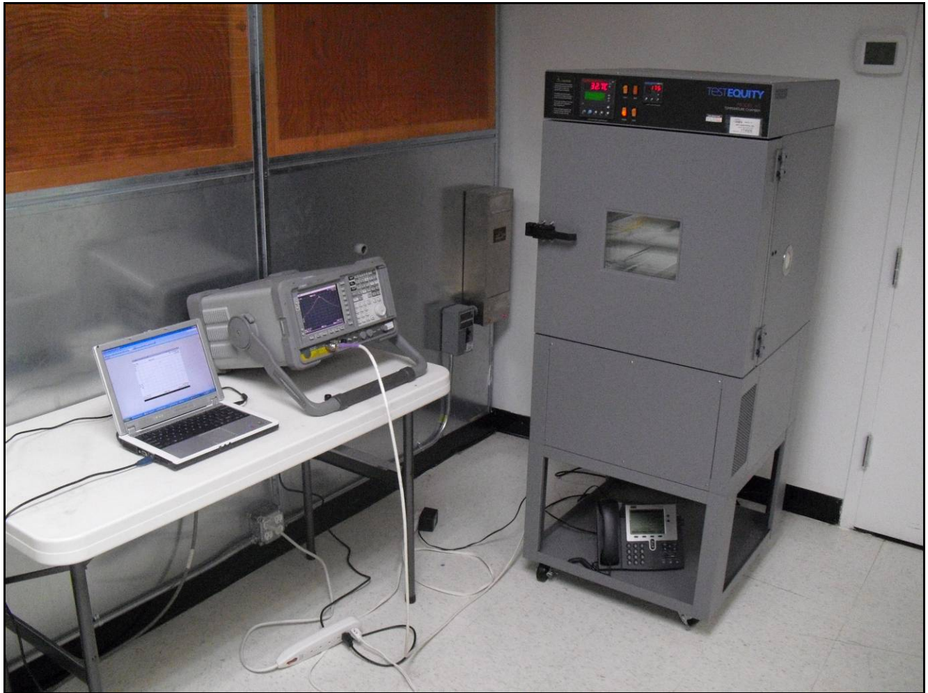
Photograph 6. Frequency Stability, Test Setup, M25 Radio
