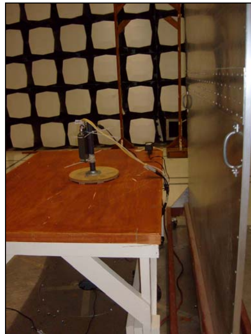
Photograph 7. Conducted Emissions, Test Setup, Side View, M5 Radio
