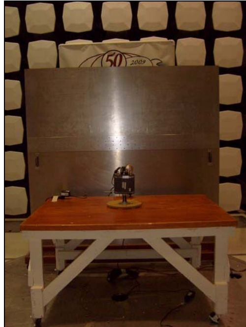
Photograph 3. Conducted Emissions, Test Setup, M25 Radio
