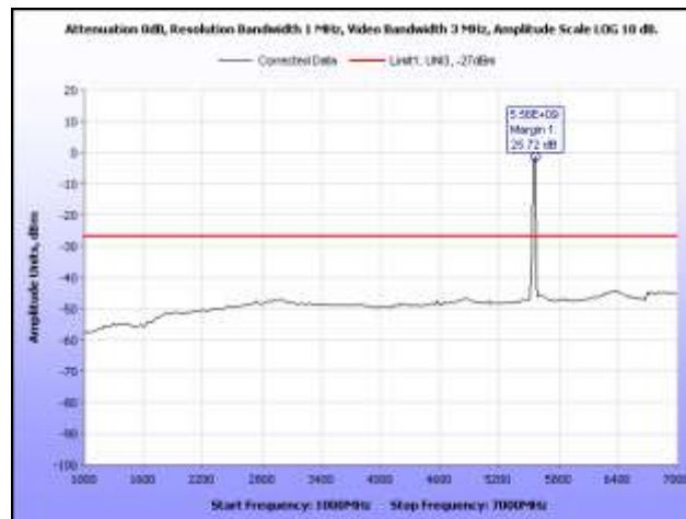
Plot 53. Radiated Spurious Emissions, 5560 MHz, 1 GHz – 7 GHz, Omni Antenna
