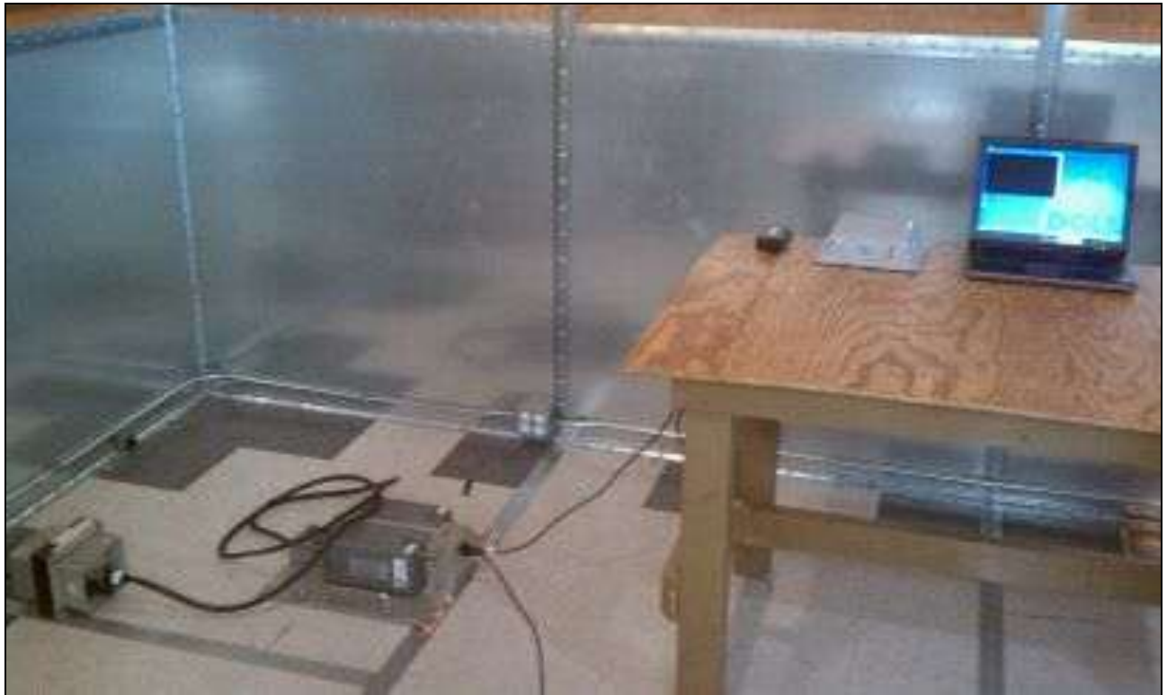
Photograph 2. Conducted Emissions, Test Setup
