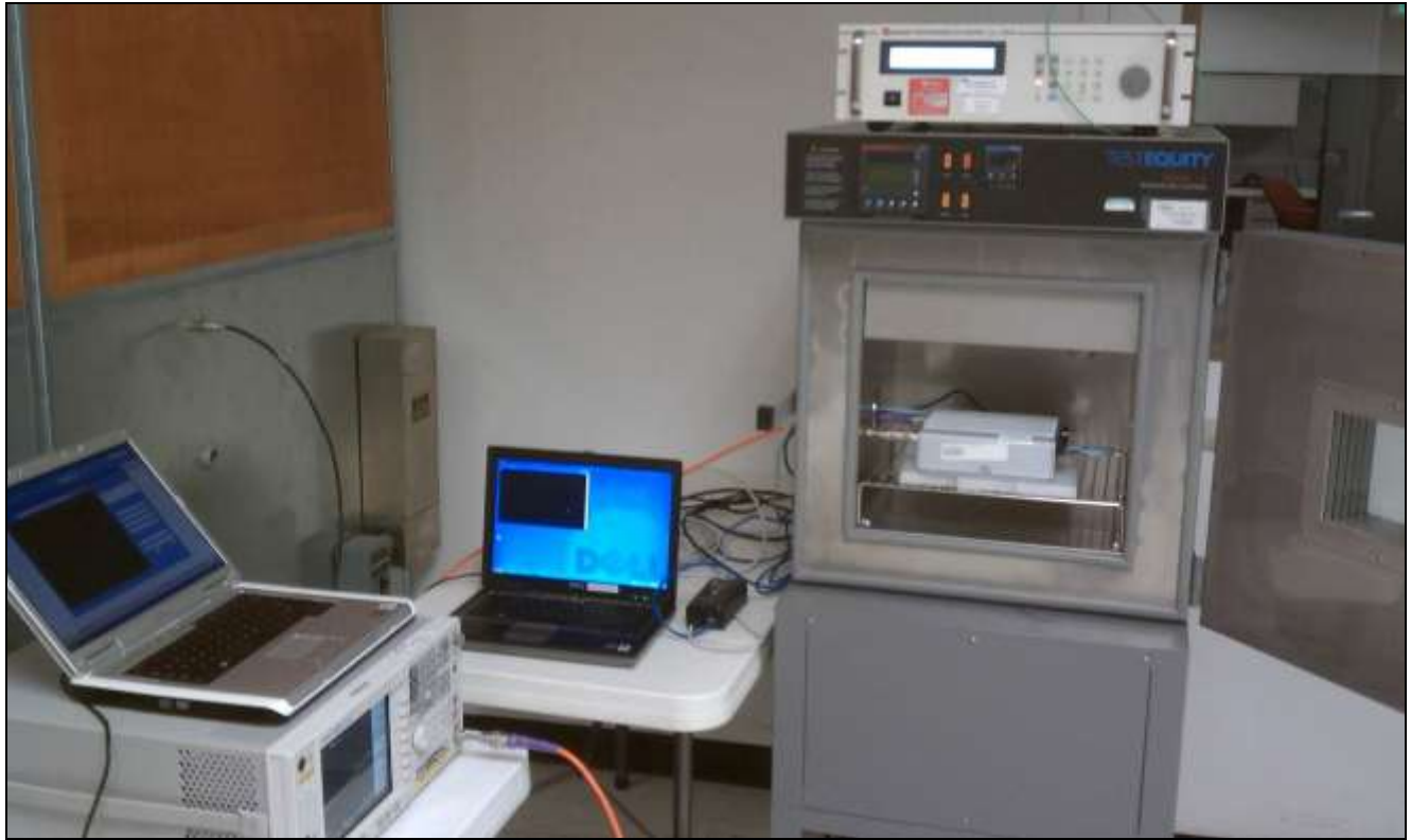
Photograph 5. Frequency Stability, Test Setup
