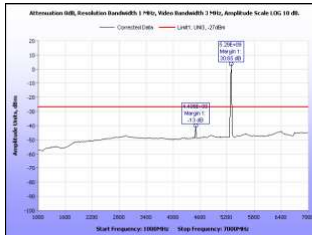
Plot 41. Radiated Spurious Emissions, 5300 MHz, 1 GHz – 7 GHz, Omni Antenna
