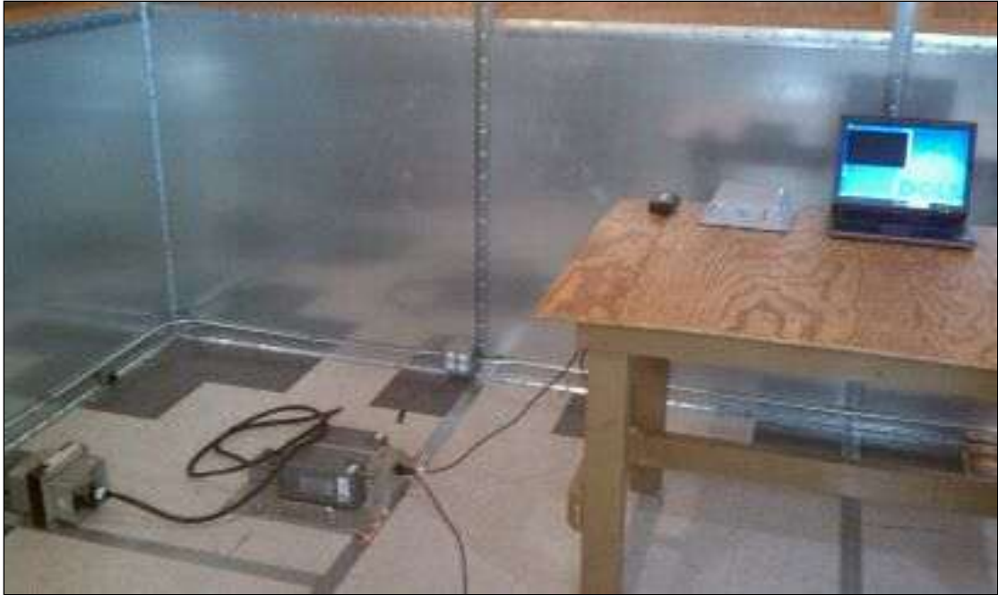
Photograph 1. Conducted Emissions, Test Setup
