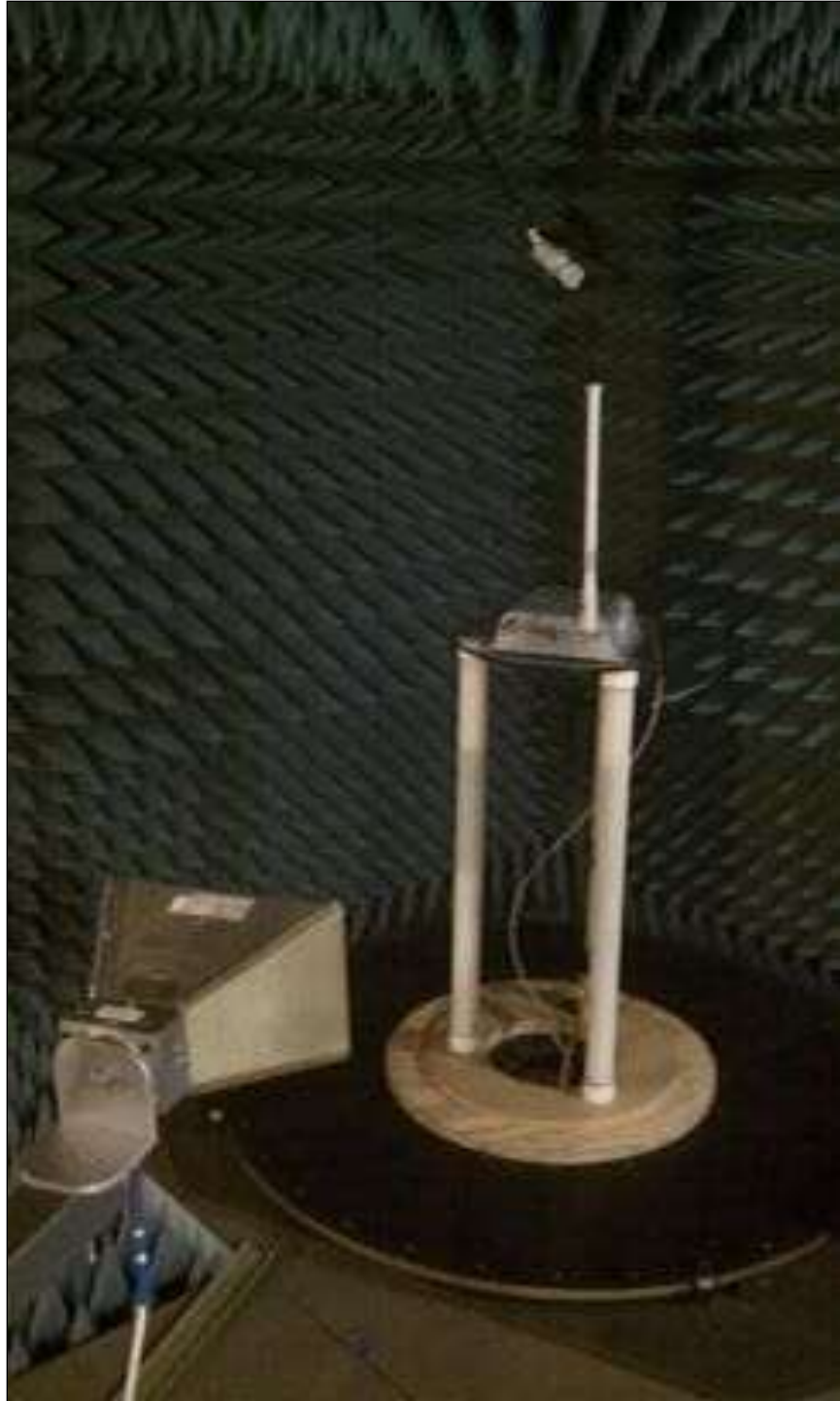
Photograph 3. Radiated Spurious Emissions, Test Setup
