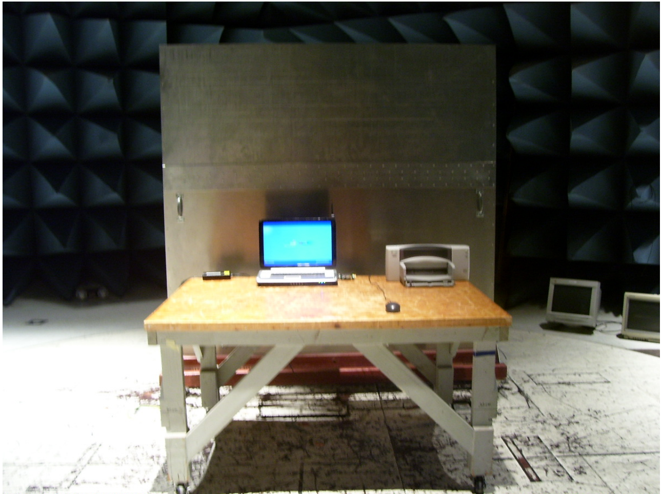
Photograph 2. Conducted Emissions Test Setup – Front View
