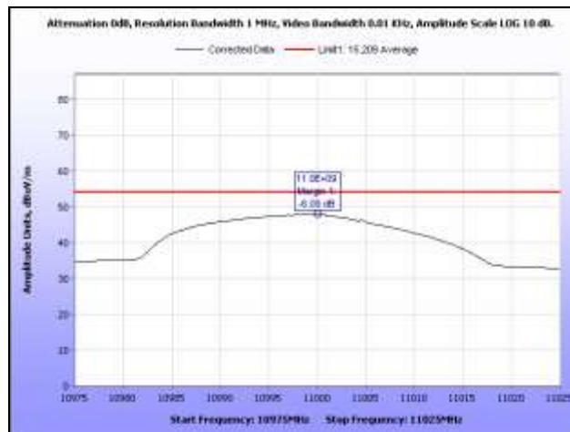
Plot 93. Radiated Spurious Emissions, 5500 MHz, 2 nd Harmonic, Average
