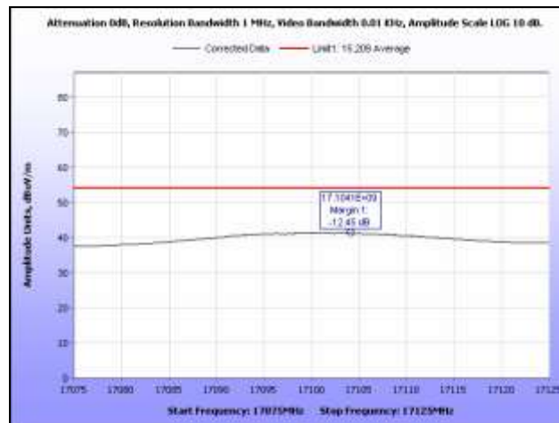
Plot 111. Radiated Spurious Emissions, 5700 MHz, 3 rd Harmonic, Average
