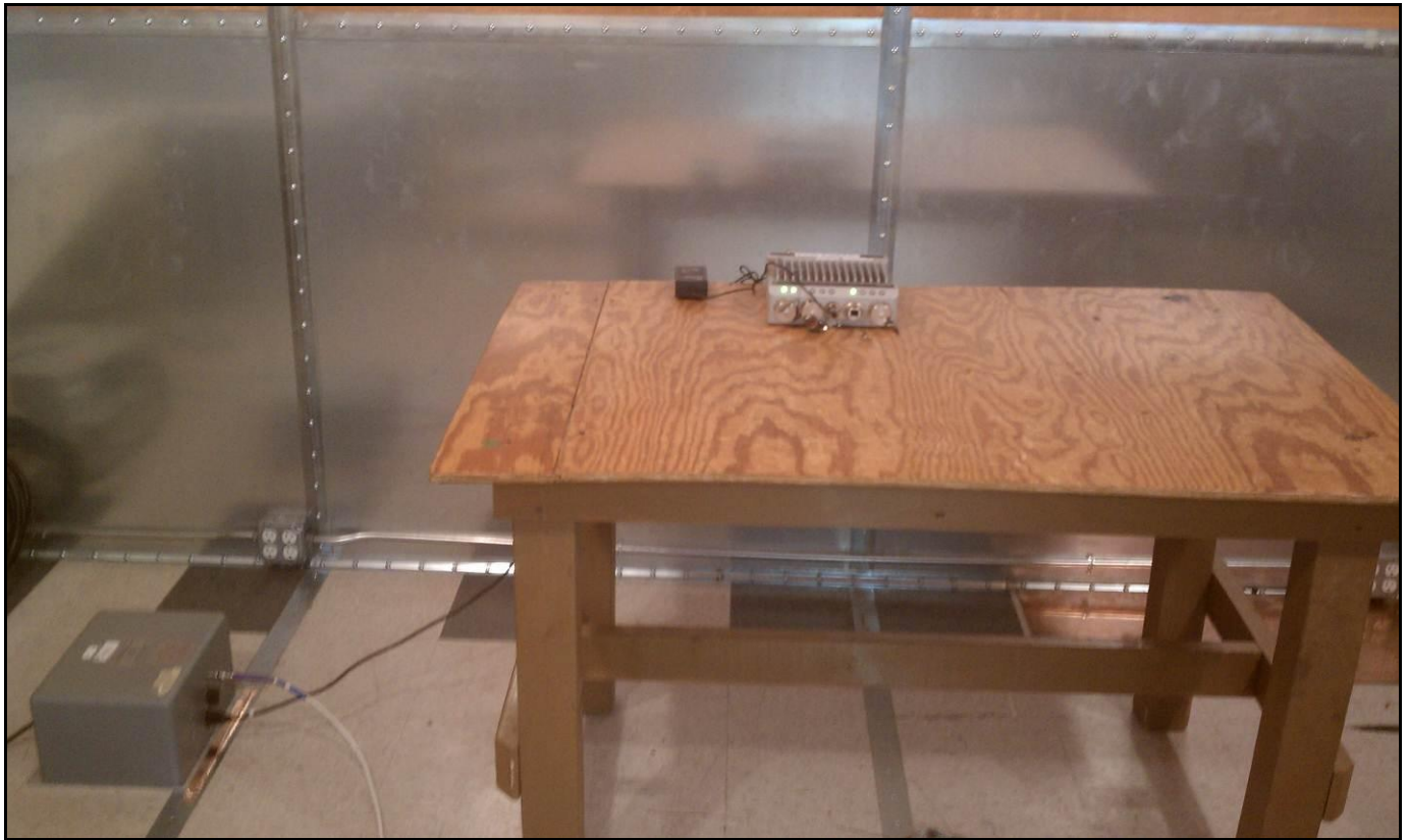
Photograph 3. §15.207 Conducted Emissions, Test Setup
