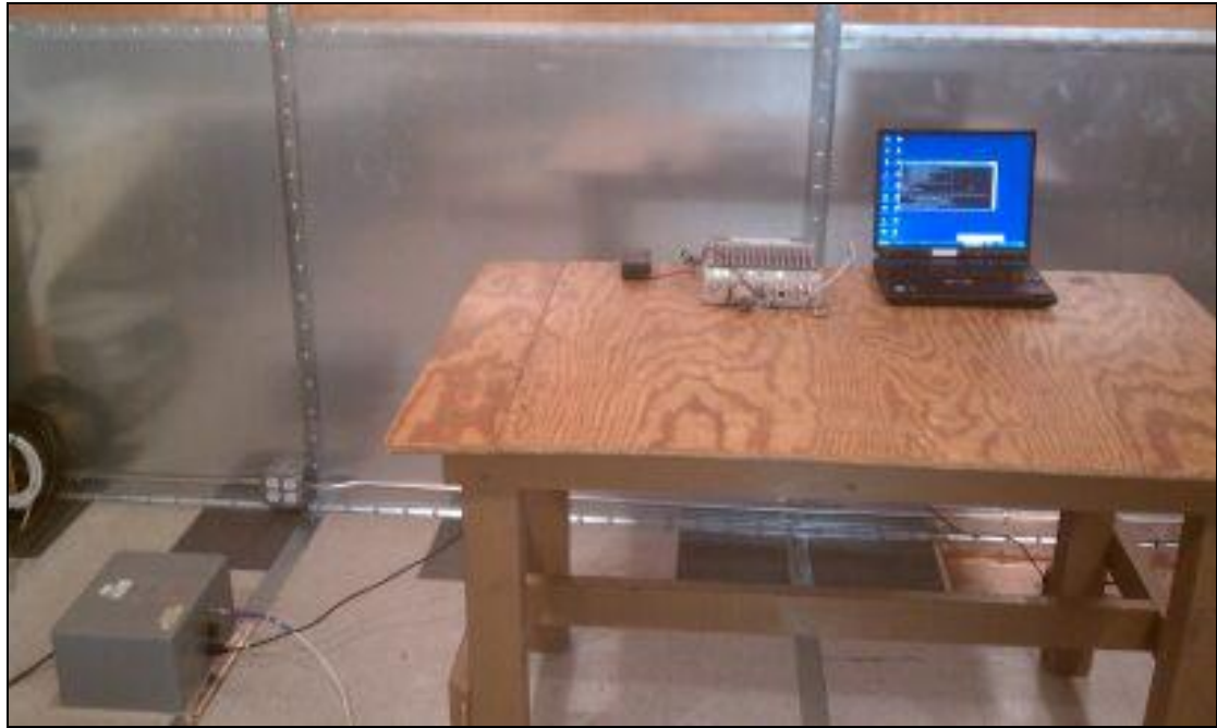
Photograph 4. Conducted Emissions, 15.207(a), Test Setup
