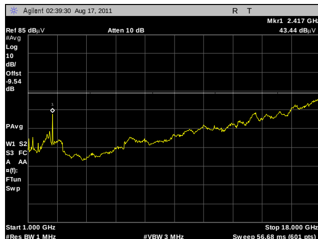
Plot 230. Radiated Spurs, Low Channel, 2.4 GHz, 802.11g HT20, 1 GHz – 18 GHz, Average, Sector
