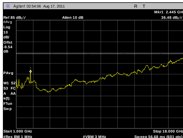
Plot 245. Radiated Spurs, Low Channel, 2.4 GHz, 802.11g HT40, 1 GHz – 18 GHz, Average, Sector
