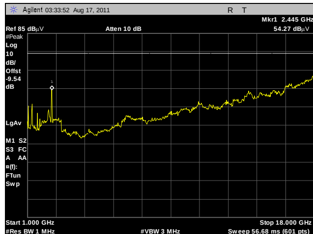
Plot 191. Radiated Spurs, Mid Channel, 2.4 GHz, 802.11g HT40, 1 GHz – 18 GHz, Peak, Omni
