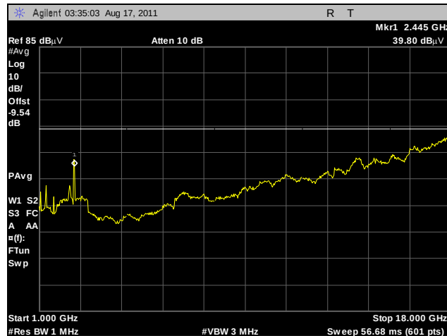
Plot 185. Radiated Spurs, Low Channel, 2.4 GHz, 802.11g HT40, 1 GHz – 18 GHz, Average, Omni
