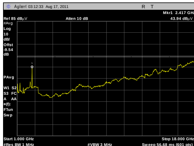
Plot 155. Radiated Spurs, Low Channel, 2.4 GHz, 802.11g, 1 GHz – 18 GHz, Average, Omni
