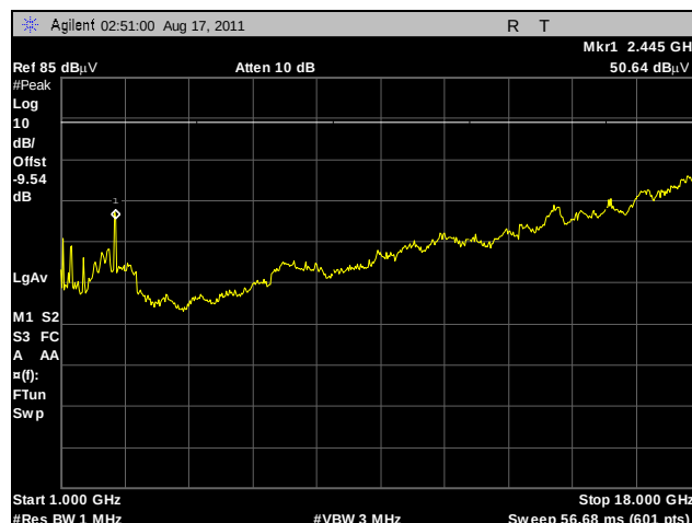
Plot 246. Radiated Spurs, Low Channel, 2.4 GHz, 802.11g HT40, 1 GHz – 18 GHz, Peak, Sector
