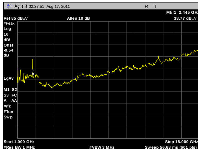
Plot 201. Radiated Spurs, Low Channel, 2.4 GHz, 802.11b, 1 GHz – 18 GHz, Peak, Sector
