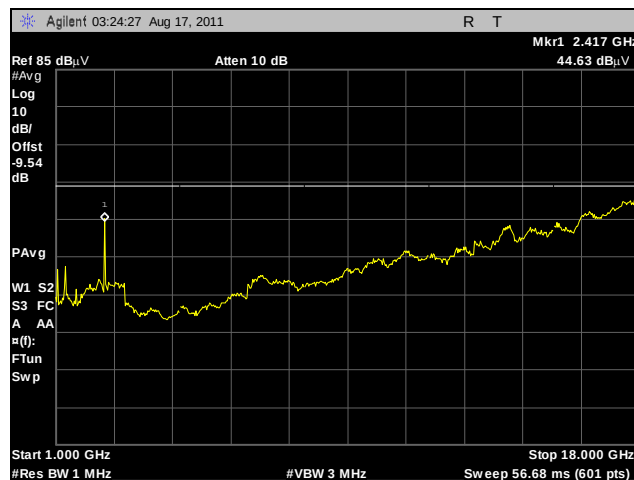
Plot 140. Radiated Spurs, Low Channel, 2.4 GHz, 802.11b, 1 GHz – 18 GHz, Average, Omni
