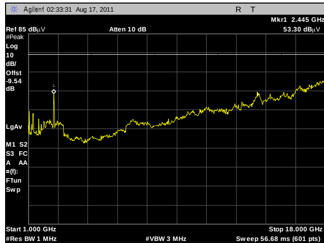
Plot 226. Radiated Spurs, High Channel, 2.4 GHz, 802.11g, 1 GHz – 18 GHz, Peak, Sector
