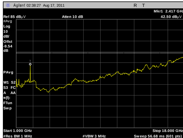
Plot 200. Radiated Spurs, Low Channel, 2.4 GHz, 802.11b, 1 GHz – 18 GHz, Average, Sector
