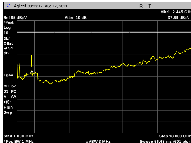
Plot 141. Radiated Spurs, Low Channel, 2.4 GHz, 802.11b, 1 GHz – 18 GHz, Peak, Omni
