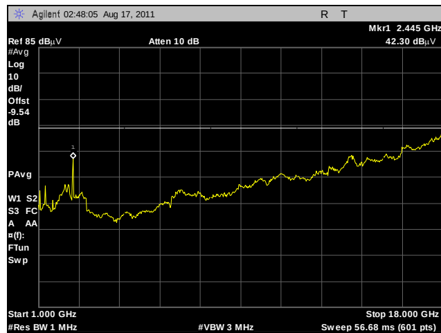
Plot 250. Radiated Spurs, Mid Channel, 2.4 GHz, 802.11g HT40, 1 GHz – 18 GHz, Average, Sector
