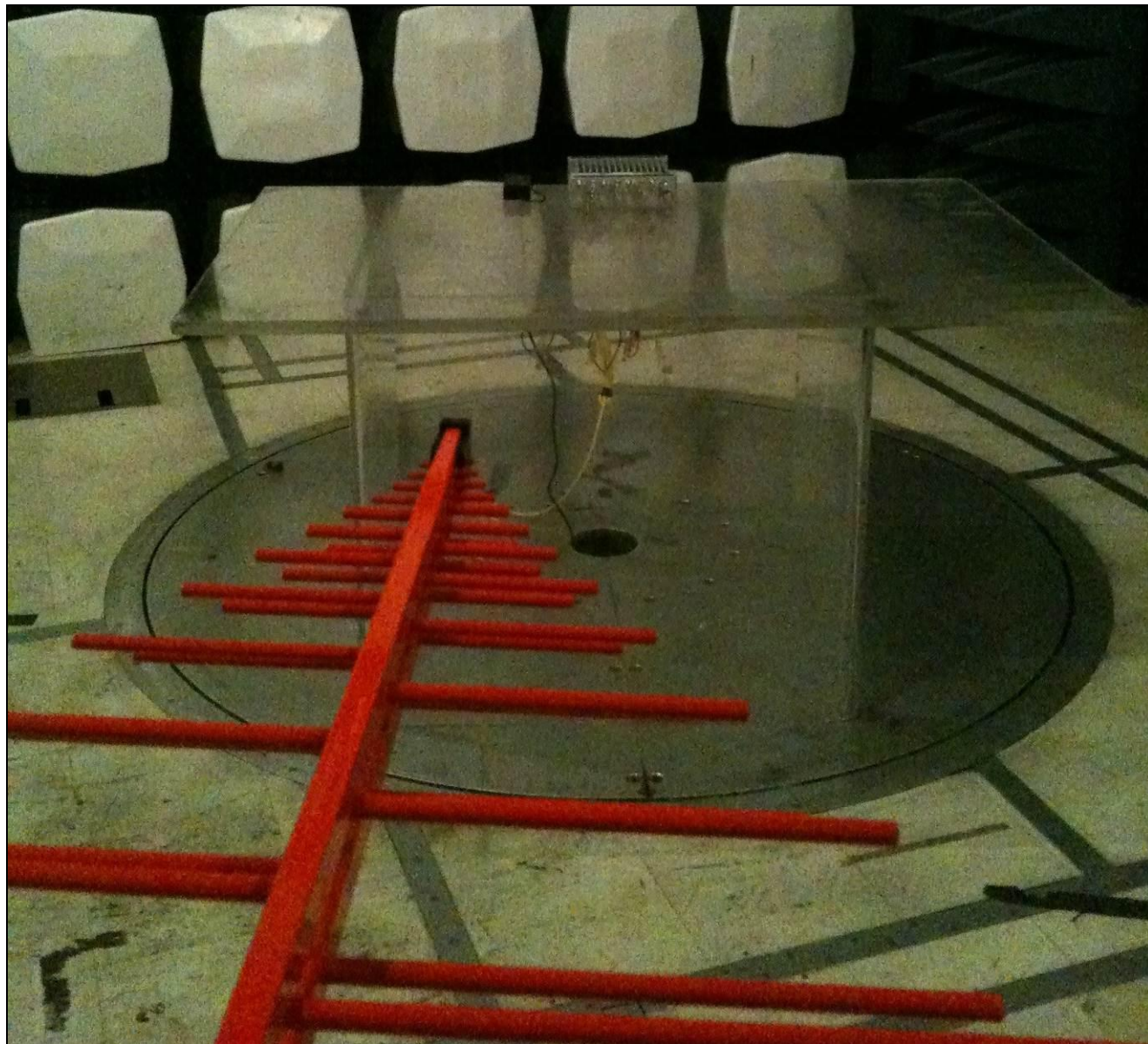
Photograph 3. Radiated Emission, Test Setup
