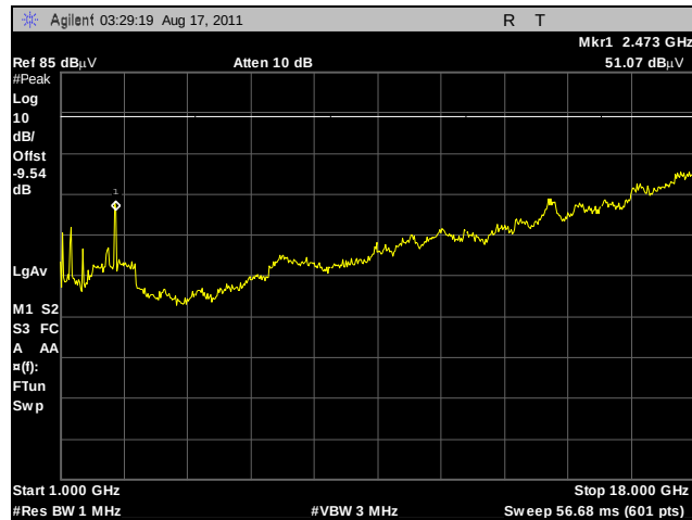
Plot 181. Radiated Spurs, High Channel, 2.4 GHz, 802.11g HT20, 1 GHz – 18 GHz, Peak, Omni
