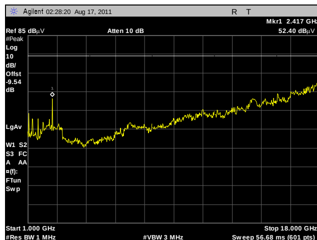
Plot 216. Radiated Spurs, Low Channel, 2.4 GHz, 802.11g, 1 GHz – 18 GHz, Peak, Sector
