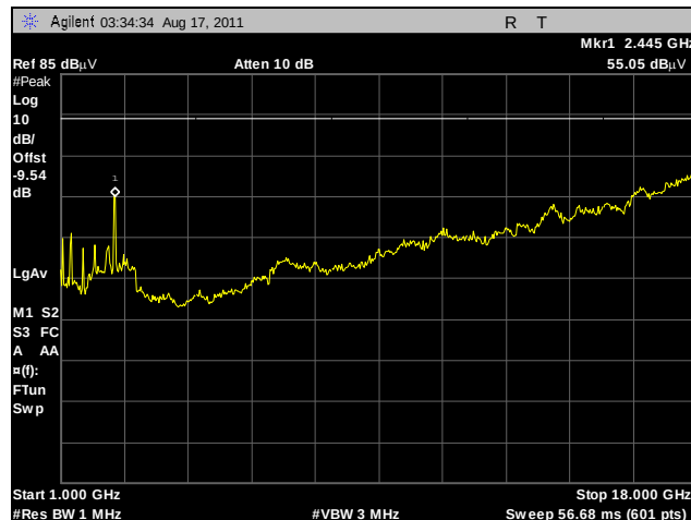
Plot 186. Radiated Spurs, Low Channel, 2.4 GHz, 802.11g HT40, 1 GHz – 18 GHz, Peak, Omni
