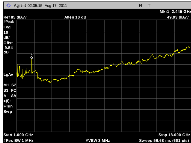
Plot 211. Radiated Spurs, High Channel, 2.4 GHz, 802.11b, 1 GHz – 18 GHz, Peak, Sector
