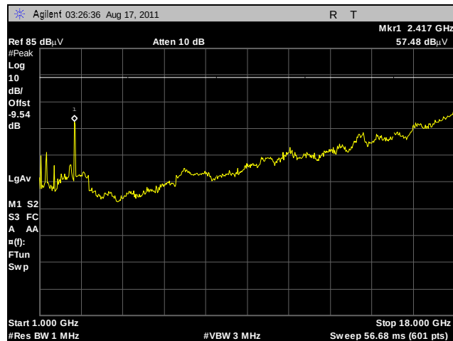
Plot 176. Radiated Spurs, Mid Channel, 2.4 GHz, 802.11g HT20, 1 GHz – 18 GHz, Peak, Omni
