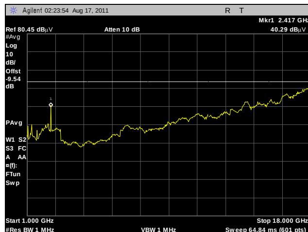
Plot 215. Radiated Spurs, Low Channel, 2.4 GHz, 802.11g, 1 GHz – 18 GHz, Average, Sector
