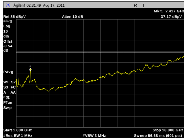
Plot 220. Radiated Spurs, Mid Channel, 2.4 GHz, 802.11g, 1 GHz – 18 GHz, Average, Sector
