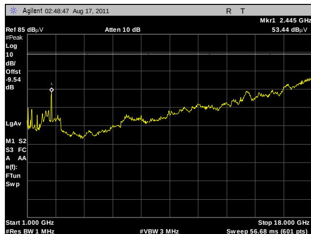
Plot 251. Radiated Spurs, Mid Channel, 2.4 GHz, 802.11g HT40, 1 GHz – 18 GHz, Peak, Sector
