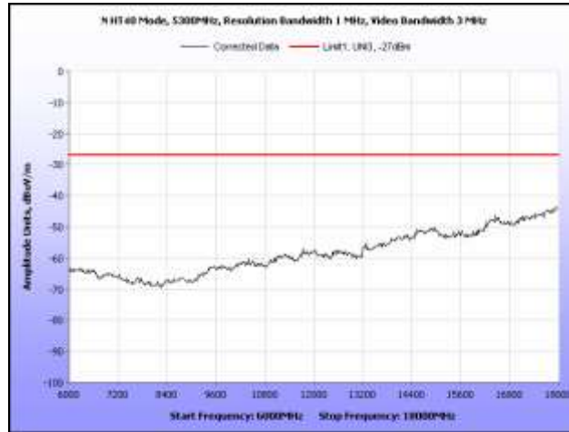
Plot 270. Radiated Spurious, 802.11n 40 MHz, 5300 MHz, 6 GHz – 18 GHz, Omni Antenna
