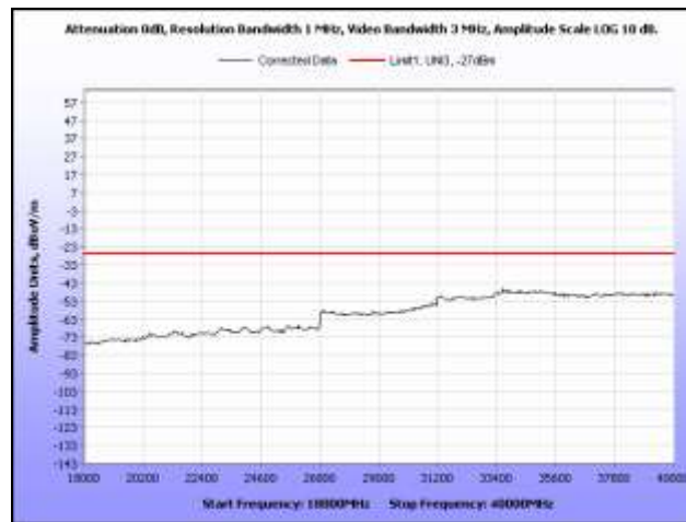
Plot 259. Radiated Spurious, 802.11n 20 MHz, 5580 MHz, 18 GHz – 40 GHz, Omni Antenna
