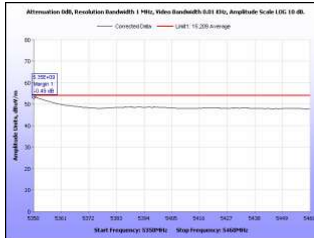
Plot 392. Restricted Band, 802.11n 40 MHz, 5310 MHz, Average, Omni Antenna
