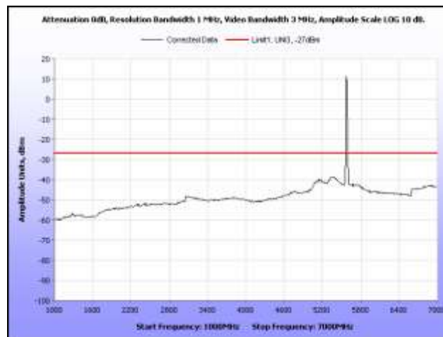
Plot 329. Radiated Spurious, 802.11n 20 MHz, 5580 MHz, 1 GHz – 7 GHz, Sector Antenna
