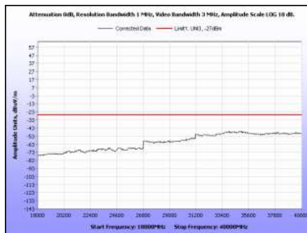
Plot 263. Radiated Spurious, 802.11n 20 MHz, 5700 MHz, 18 GHz – 40 GHz, Omni Antenna
