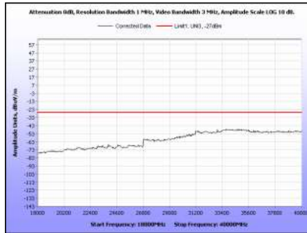
Plot 231. Radiated Spurious, 802.11a, 5500 MHz, 18 MHz – 40 GHz, Omni Antenna
