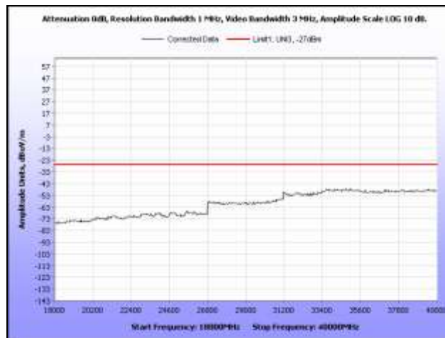
Plot 295. Radiated Spurious, 802.11a, 5300 MHz, 18 GHz – 40 GHz, Sector Antenna
