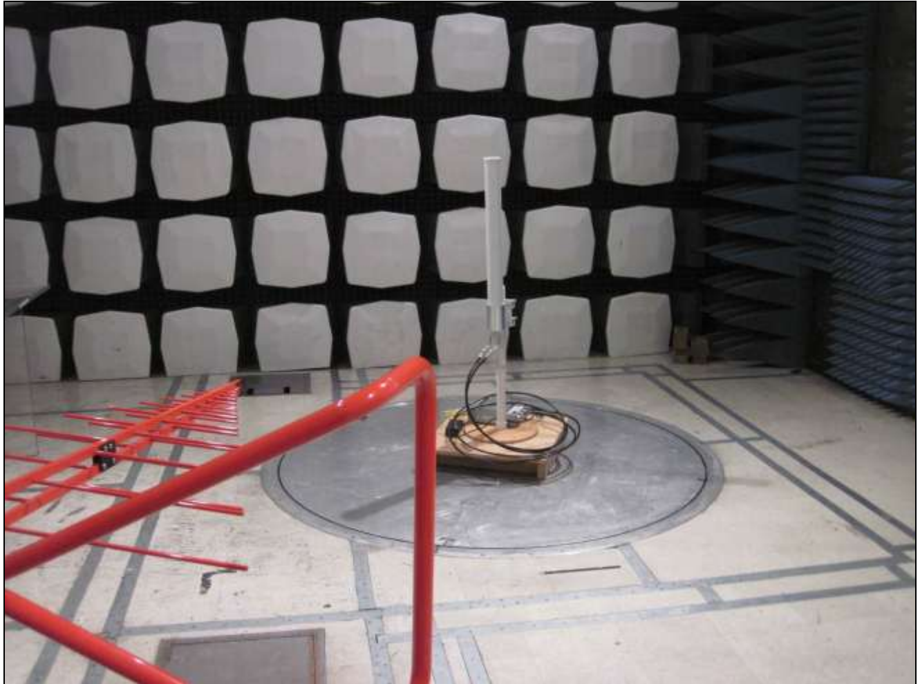
Photograph 2. Radiated Emission, Test Setup
