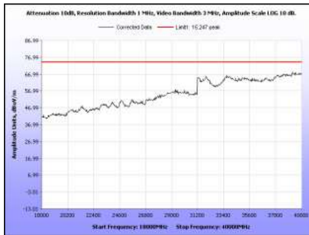
Plot 342. Radiated Spurs, Mid Channel, 5.8 GHz, 802.11n 20 MHz, 18 GHz – 40 GHz, Peak, Sector
