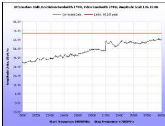
Plot 354. Radiated Spurs, Low Channel, 5.8 GHz, 802.11n 40 MHz, 18 GHz – 40 GHz, Peak, Sector
