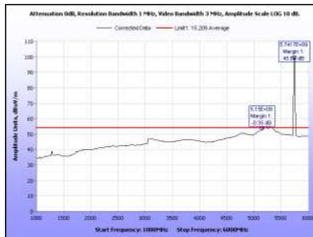
Plot 332. Radiated Spurs, Low Channel, 5.8 GHz, 802.11n 20 MHz, 1 GHz – 6 GHz, Average, Sector
