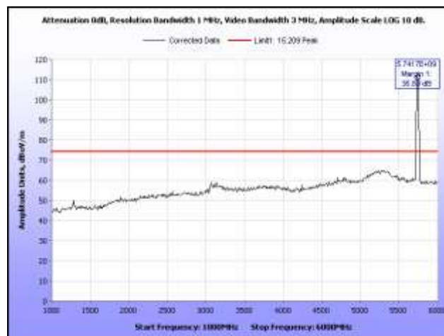
Plot 333. Radiated Spurs, Low Channel, 5.8 GHz, 802.11n 20 MHz, 1 GHz – 6 GHz, Peak, Sector
