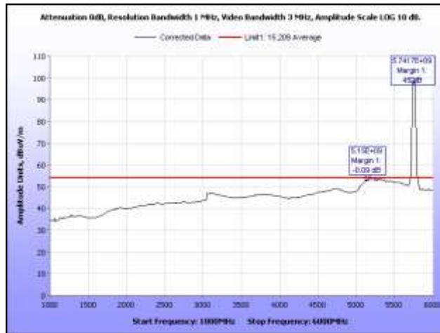
Plot 296. Radiated Spurs, Low Channel, 5.8 GHz, 802.11n 40 MHz, 1 GHz – 6 GHz, Average, Omni
