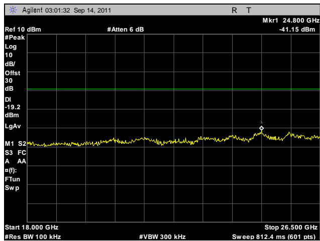
Plot 428. Conducted Spurious Emissions, Mid Channel, 2.4 GHz, 802.11g HT20, Port B, 18 GHz – 26.5 GHz
