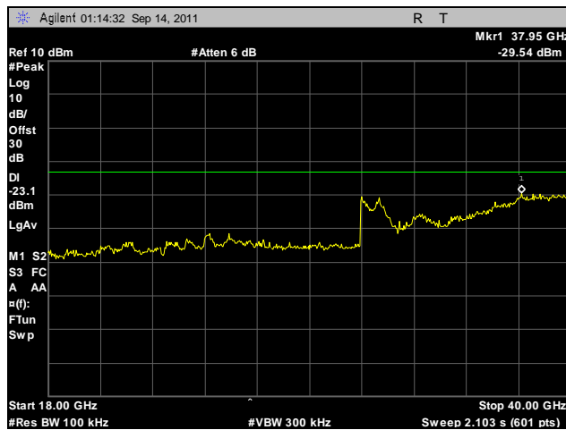
Plot 485. Conducted Spurious Emissions, Low Channel, 5.8 GHz, 802.11n 40 MHz, Port B, 18 GHz – 40 GHz
