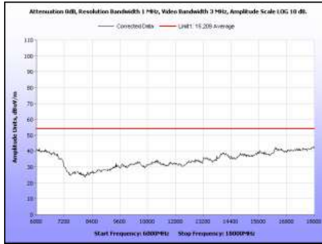
Plot 310. Radiated Spurs, High Channel, 5.8 GHz, 802.11n 40 MHz, 6 GHz – 18 GHz, Peak under Avg., Omni
