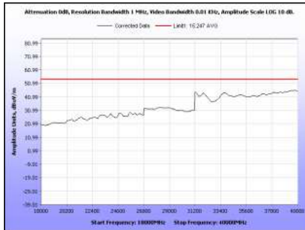
Plot 341. Radiated Spurs, Mid Channel, 5.8 GHz, 802.11n 20 MHz, 18 GHz – 40 GHz, Average, Sector
