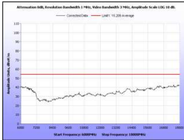
Plot 292. Radiated Spurs, High Channel, 5.8 GHz, 802.11n 20 MHz, 6 GHz – 18 GHz, Peak under Avg., Omni
