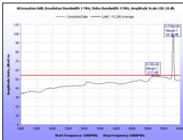
Plot 302. Radiated Spurs, Mid Channel, 5.8 GHz, 802.11n 40 MHz, 1 GHz – 6 GHz, Average, Omni
