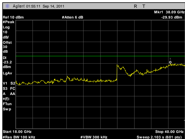
Plot 464. Conducted Spurious Emissions, Low Channel, 5.8 GHz, 802.11n 20 MHz, Port A, 18 GHz – 40 GHz
