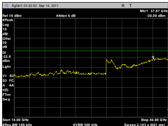
Plot 482. Conducted Spurious Emissions, Low Channel, 5.8 GHz, 802.11n 40 MHz, Port A, 18 GHz – 40 GHz
