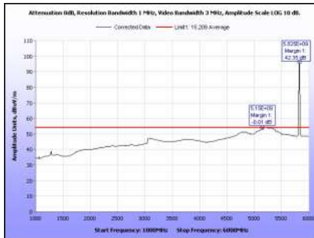
Plot 344. Radiated Spurs, High Channel, 5.8 GHz, 802.11n 20 MHz, 1 GHz – 6 GHz, Average, Sector
