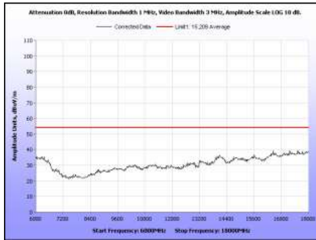
Plot 364. Radiated Spurs, High Channel, 5.8 GHz, 802.11n 40 MHz, 6 GHz – 18 GHz, Peak under Avg., Sector
