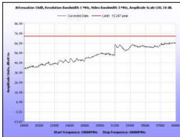
Plot 336. Radiated Spurs, Low Channel, 5.8 GHz, 802.11n 20 MHz, 18 GHz – 40 GHz, Peak, Sector
