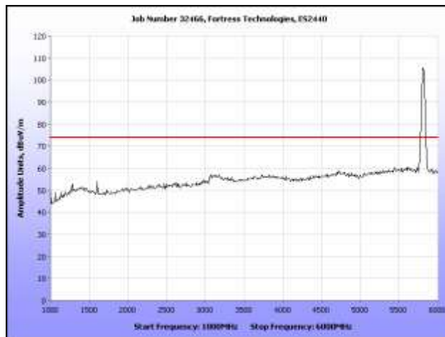
Plot 309. Radiated Spurs, High Channel, 5.8 GHz, 802.11n 40 MHz, 1 GHz – 6 GHz, Peak, Omni
