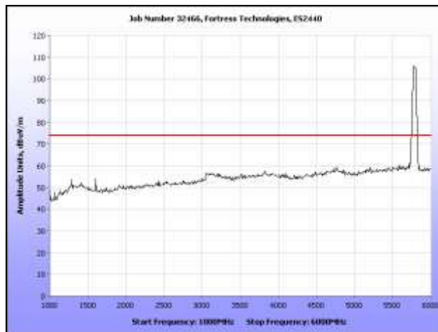
Plot 303. Radiated Spurs, Mid Channel, 5.8 GHz, 802.11n 40 MHz, 1 GHz – 6 GHz, Peak, Omni
