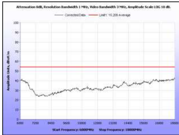
Plot 340. Radiated Spurs, Mid Channel, 5.8 GHz, 802.11n 20 MHz, 6 GHz – 18 GHz, Peak under Avg., Sector
