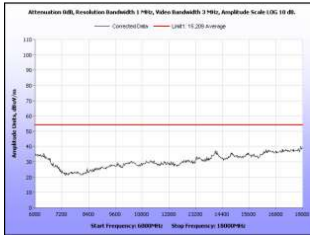
Plot 328. Radiated Spurs, High Channel, 5.8 GHz, 802.11a, 6 GHz – 18 GHz, Peak under Avg., Sector
