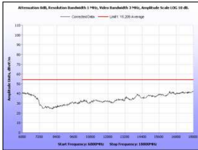
Plot 298. Radiated Spurs, Low Channel, 5.8 GHz, 802.11n 40 MHz, 6 GHz – 18 GHz, Peak under Avg., Omni
