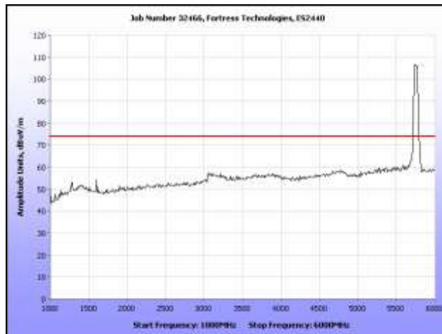
Plot 297. Radiated Spurs, Low Channel, 5.8 GHz, 802.11n 40 MHz, 1 GHz – 6 GHz, Peak, Omni
