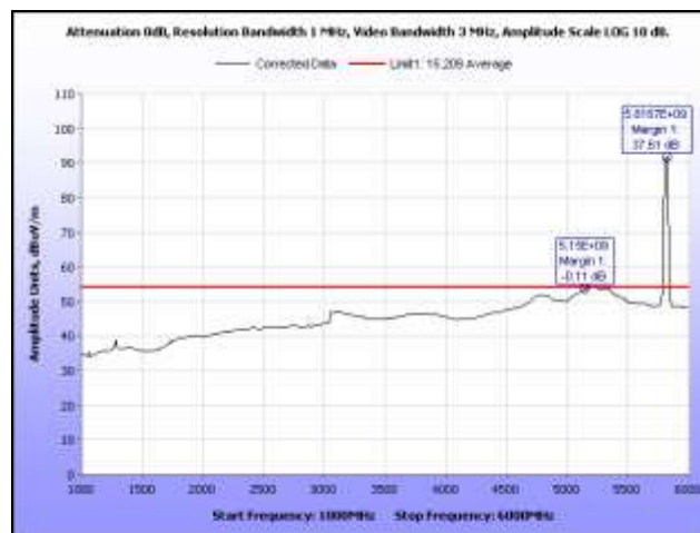
Plot 362. Radiated Spurs, High Channel, 5.8 GHz, 802.11n 40 MHz, 1 GHz – 6 GHz, Average, Sector
