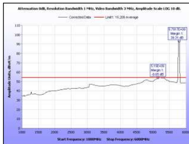
Plot 356. Radiated Spurs, Mid Channel, 5.8 GHz, 802.11n 40 MHz, 1 GHz – 6 GHz, Average, Sector
