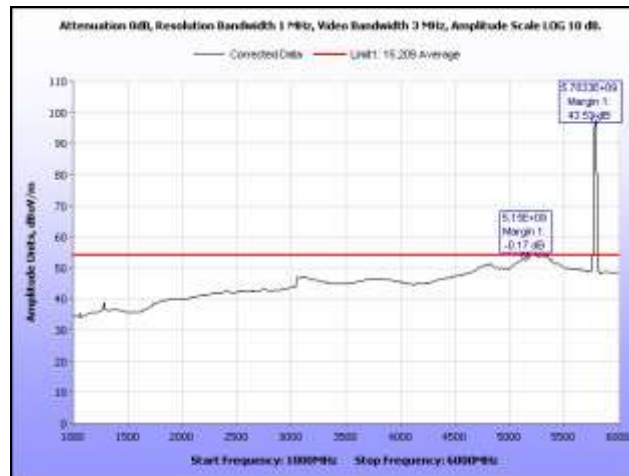
Plot 338. Radiated Spurs, Mid Channel, 5.8 GHz, 802.11n 20 MHz, 1 GHz – 6 GHz, Average, Sector
