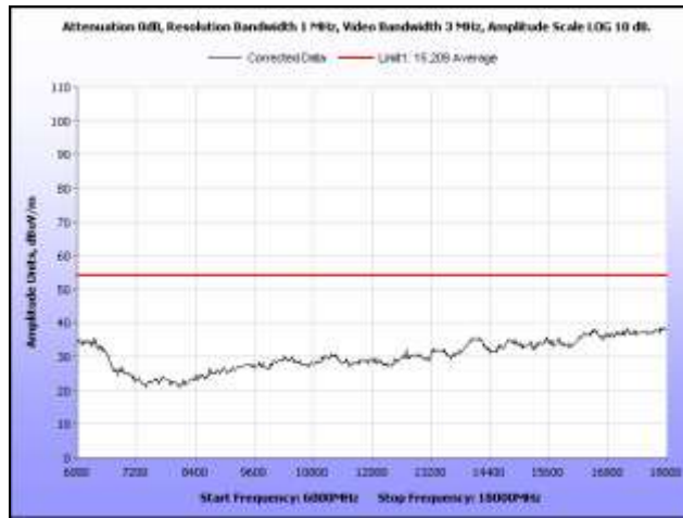
Plot 358. Radiated Spurs, Mid Channel, 5.8 GHz, 802.11n 40 MHz, 6 GHz – 18 GHz, Peak under Avg., Sector
