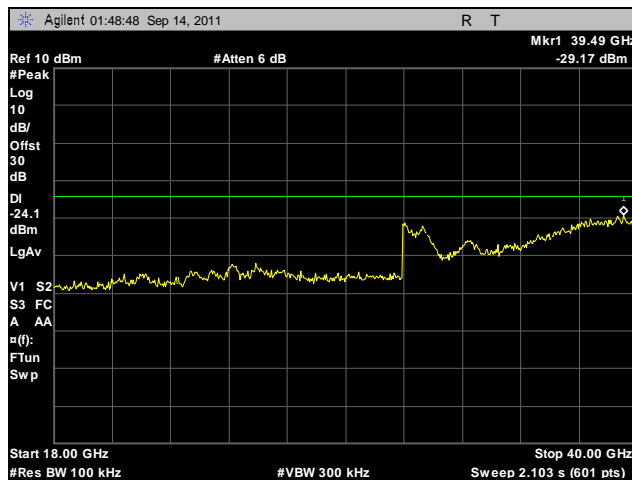
Plot 488. Conducted Spurious Emissions, Mid Channel, 5.8 GHz, 802.11n 40 MHz, Port A, 18 GHz – 40 GHz
