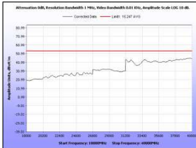
Plot 353. Radiated Spurs, Low Channel, 5.8 GHz, 802.11n 40 MHz, 18 GHz – 40 GHz, Average, Sector
