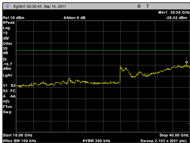
Plot 404. Conducted Spurious Emissions, Mid Channel, 2.4 GHz, 802.11b, Port A, 18 GHz – 40 GHz
