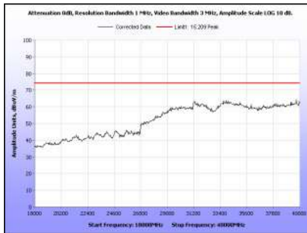
Plot 294. Radiated Spurs, High Channel, 5.8 GHz, 802.11n 20 MHz, 18 GHz – 40 GHz, Peak, Omni
