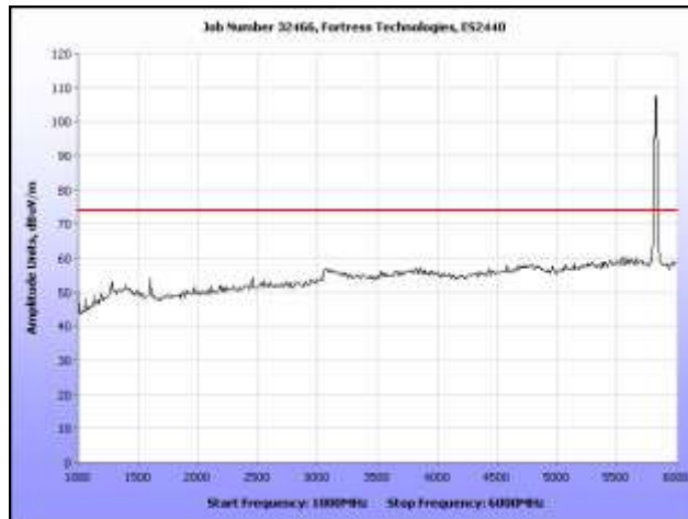
Plot 291. Radiated Spurs, High Channel, 5.8 GHz, 802.11n 20 MHz, 1 GHz – 6 GHz, Peak, Omni
