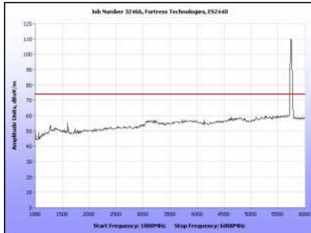
Plot 279. Radiated Spurs, Low Channel, 5.8 GHz, 802.11n 20 MHz, 1 GHz – 6 GHz, Peak, Omni
