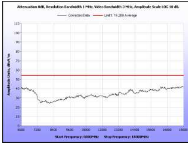
Plot 268. Radiated Spurs, Mid Channel, 5.8 GHz, 802.11a, 6 GHz – 18 GHz, Peak under Avg., Omni
