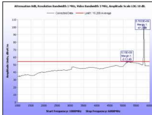
Plot 284. Radiated Spurs, Mid Channel, 5.8 GHz, 802.11n 20 MHz, 1 GHz – 6 GHz, Average, Omni
