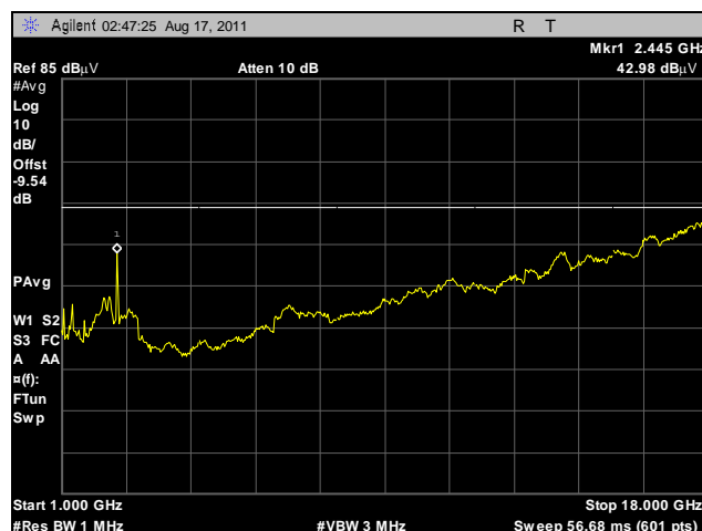
Plot 255. Radiated Spurs, High Channel, 2.4 GHz, 802.11g HT40, 1 GHz – 18 GHz, Average, Sector
