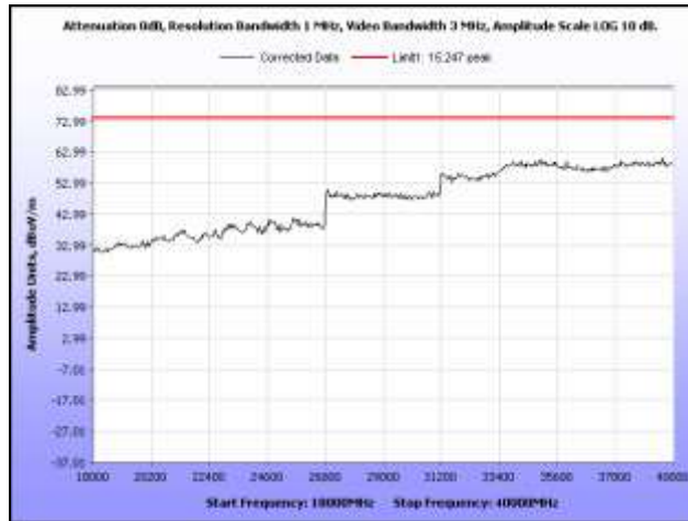
Plot 188. Radiated Spurs, Low Channel, 2.4 GHz, 802.11g HT40, 18 GHz – 40 GHz, Peak, Omni
