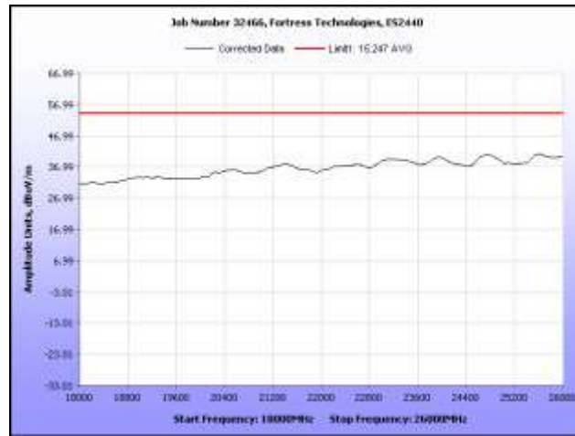
Plot 247. Radiated Spurs, Low Channel, 2.4 GHz, 802.11g HT40, 18 GHz – 26 GHz, Average, Sector
