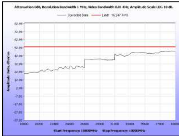
Plot 187. Radiated Spurs, Low Channel, 2.4 GHz, 802.11g HT40, 18 GHz – 40 GHz, Average, Omni
