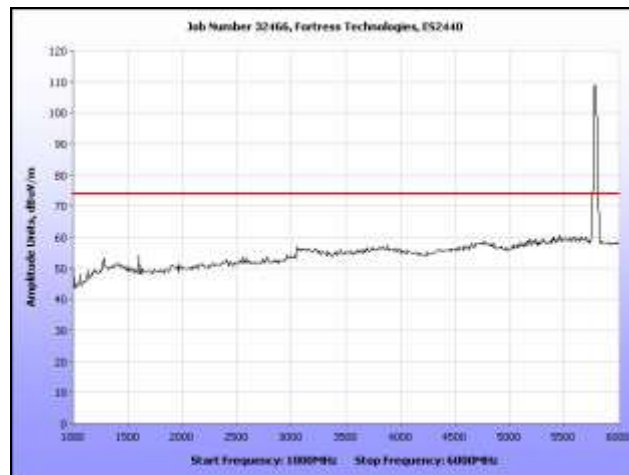
Plot 285. Radiated Spurs, Mid Channel, 5.8 GHz, 802.11n 20 MHz, 1 GHz – 6 GHz, Peak, Omni
