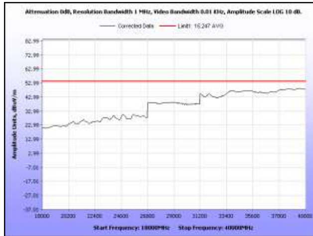
Plot 182. Radiated Spurs, High Channel, 2.4 GHz, 802.11g HT20, 18 GHz – 40 GHz, Average, Omni
