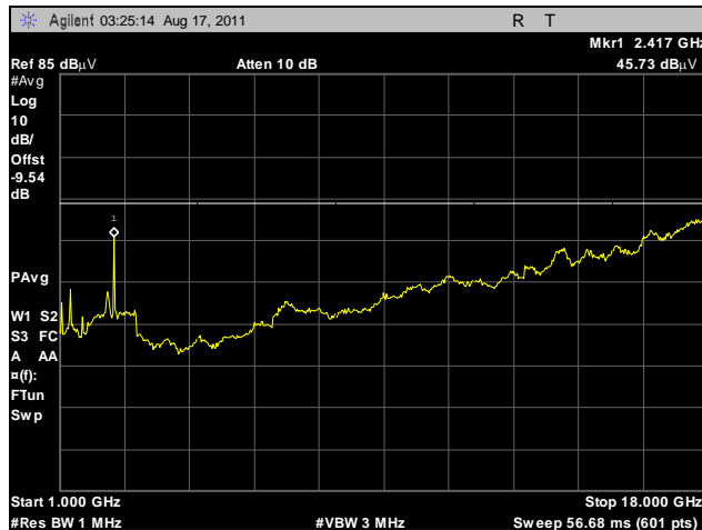
Plot 170. Radiated Spurs, Low Channel, 2.4 GHz, 802.11g HT20, 1 GHz – 18 GHz, Average, Omni
