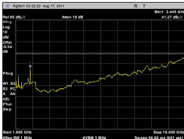
Plot 195. Radiated Spurs, High Channel, 2.4 GHz, 802.11g HT40, 1 GHz – 18 GHz, Average, Omni
