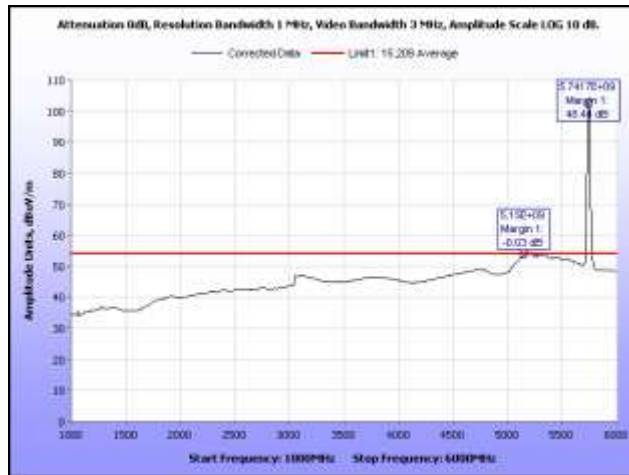
Plot 278. Radiated Spurs, Low Channel, 5.8 GHz, 802.11n 20 MHz, 1 GHz – 6 GHz, Average, Omni
