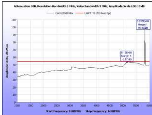
Plot 290. Radiated Spurs, High Channel, 5.8 GHz, 802.11n 20 MHz, 1 GHz – 6 GHz, Average, Omni
