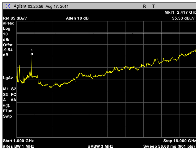
Plot 171. Radiated Spurs, Low Channel, 2.4 GHz, 802.11g HT20, 1 GHz – 18 GHz, Peak, Omni
