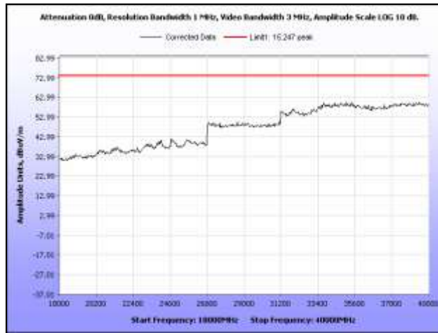
Plot 193. Radiated Spurs, Mid Channel, 2.4 GHz, 802.11g HT40, 18 GHz – 40 GHz, Peak, Omni
