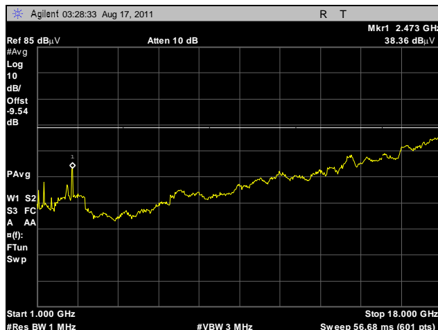
Plot 180. Radiated Spurs, High Channel, 2.4 GHz, 802.11g HT20, 1 GHz – 18 GHz, Average, Omni
