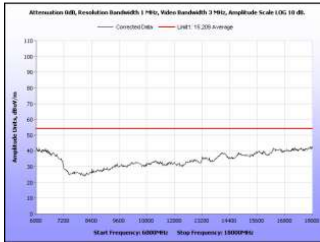
Plot 262. Radiated Spurs, Low Channel, 5.8 GHz, 802.11a, 6 GHz – 18 GHz, Peak under Avg., Omni
