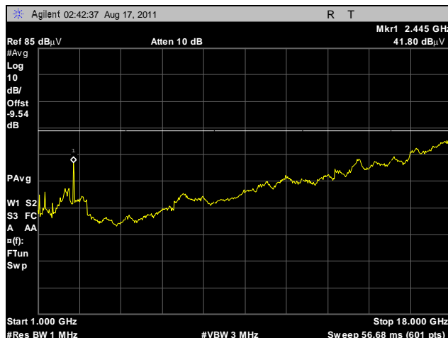
Plot 240. Radiated Spurs, High Channel, 2.4 GHz, 802.11g HT20, 1 GHz – 18 GHz, Average, Sector
