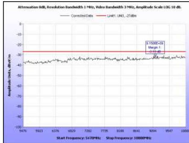
Plot 48. Radiated Spurious Emissions, 5300 MHz, HT20, 5.47 GHz – 10 GHz
