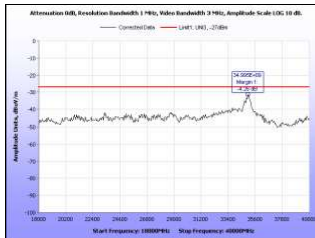
Plot 41. Radiated Spurious Emissions, 5260 MHz, HT20, 18 GHz – 40 GHz
