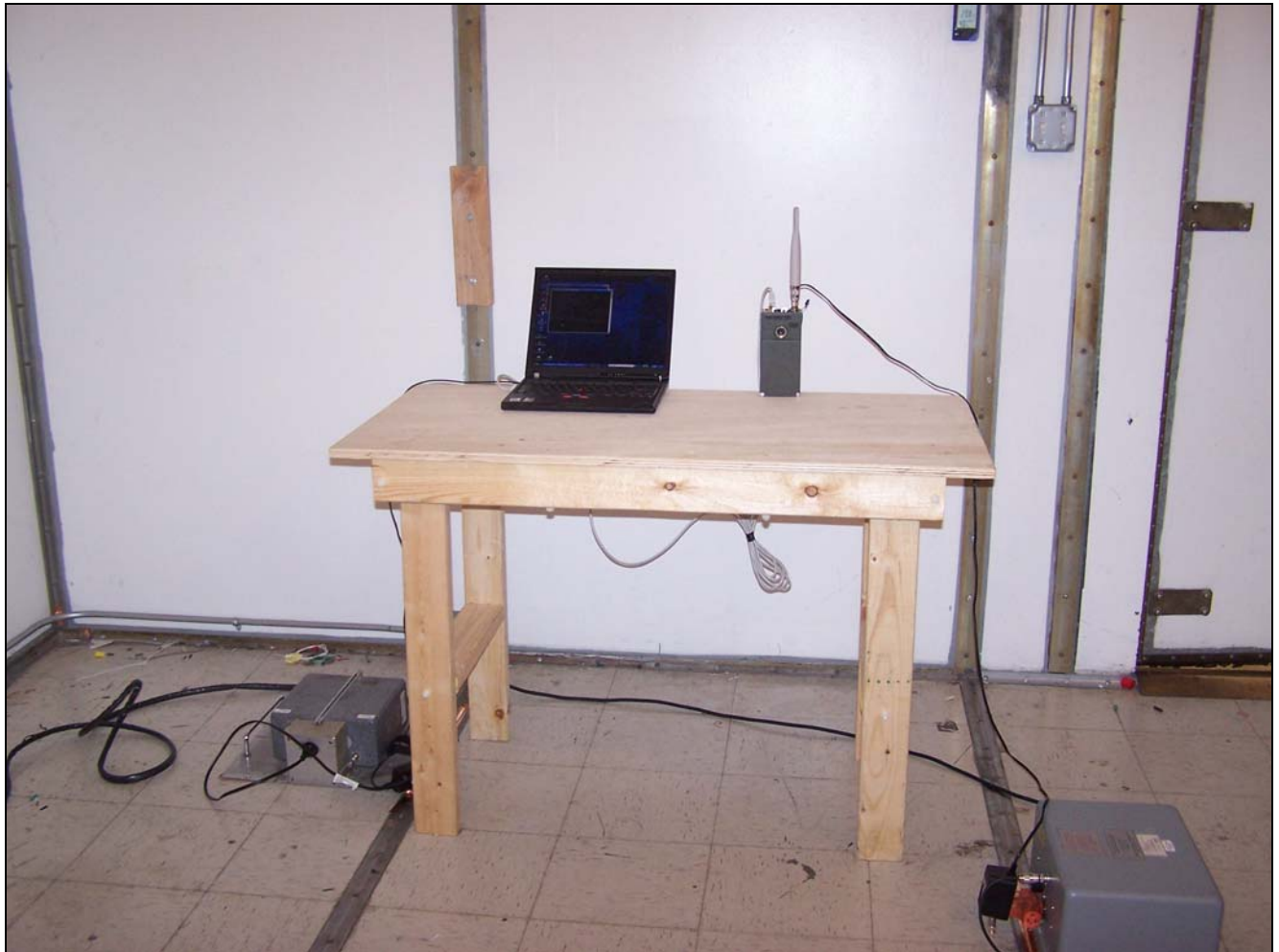
Photograph 2. Conducted Emissions, Test Setup
