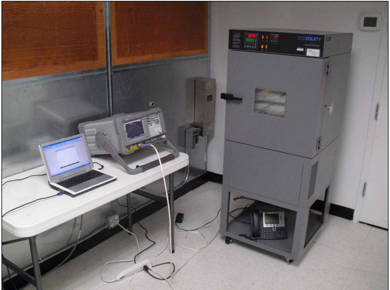
Photograph 3. Frequency Stability, Test Setup
