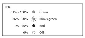
\* When the battery level is low, the front derailleur stops operating first, and then the rear derailleur. When the battery is completely drained, the derailleurs are fixed at the last gear position. It is recommended to charge the battery as soon as possible when the LED lights red.
