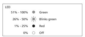
\* When the battery level is low, the front derailleur stops operating first, and then the rear derailleur. When the battery is completely drained, the derailleurs are fixed at the last gear position. It is recommended to charge the battery as soon as possible when the LED lights red.
