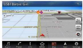
The 3D map is a map screen using a viewing position above the vehicle while looking in the direction of the car heading. It is suitable for understanding the image of the direction, because the perspective of the travelling direction can be adjusted as required.
