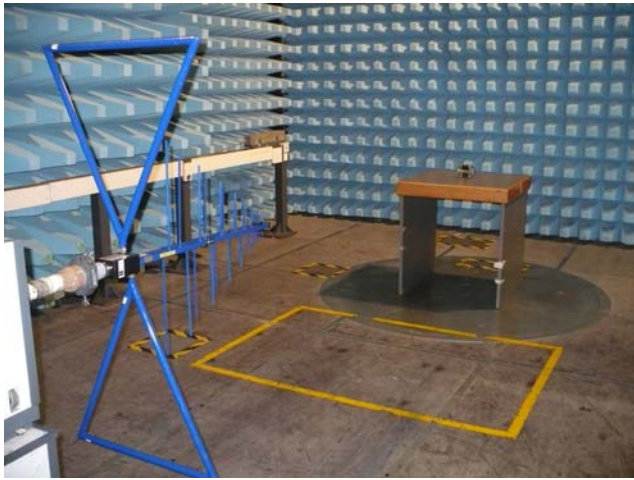
PHOTO 2 – SET-UP FOR EMISSION RADIATED TEST
