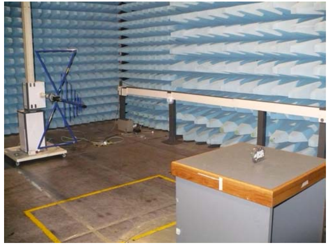
PHOTO 2 – SET-UP FOR EMISSION RADIATED TEST
