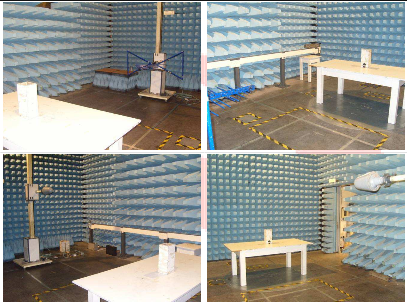
PHOTO 2 – RADIATED EMISSION SETUP
