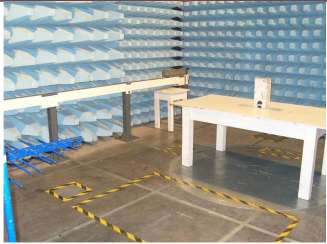
PHOTO 2 – RADIATED EMISSION SETUP
