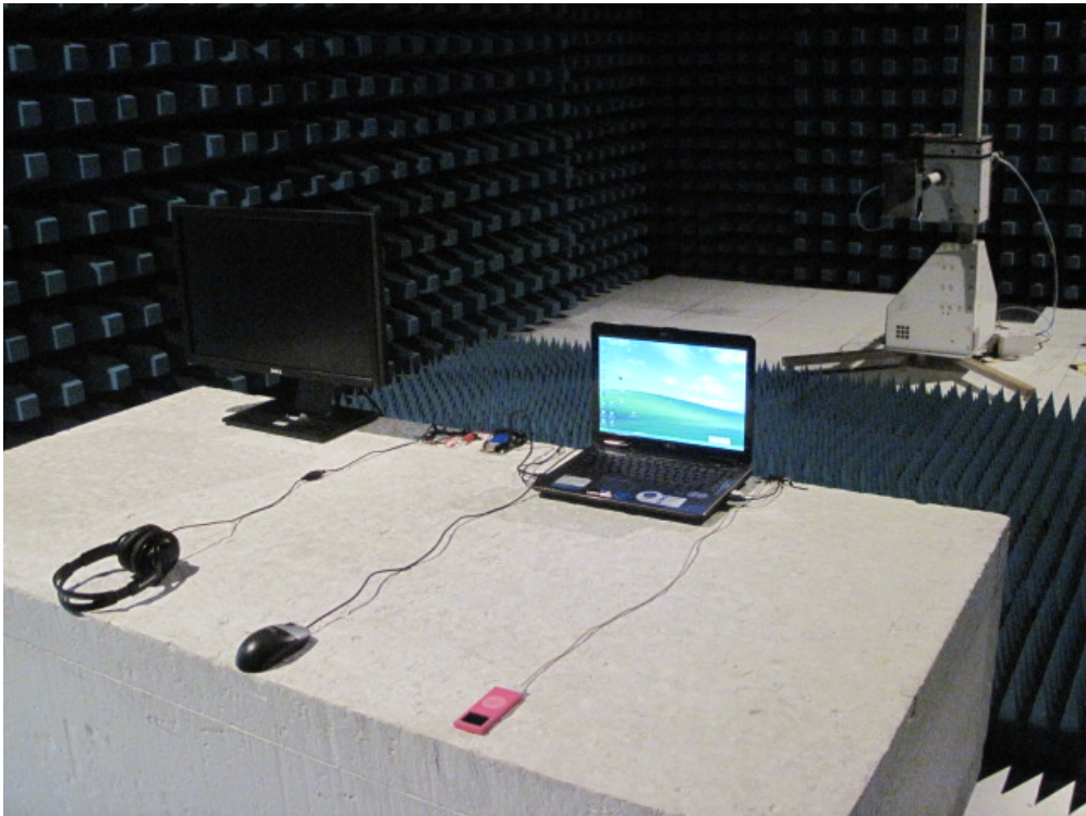
Description: Front View of Radiated Emission Test Setup for Above 1GHz-Mode 1~2
