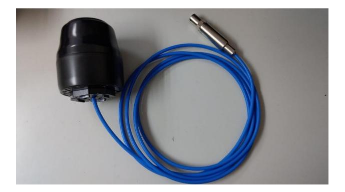
A set of three "D" cells are enclosed that power the electronics and the Cellular modem. The TM1 utilizes the LTE CAT M1 service provided by Verizon Wireless in the USA that operates in the 750 MHz cellular 4G band.
