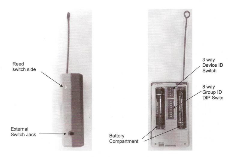
Transmitter is put in a small plastic casing with a LED indicator. The LED flash after power on, indicating that it is operating. Transmitter operates with two AA-size batteries. Group ID and Device ID allow user to select an unique ID.
