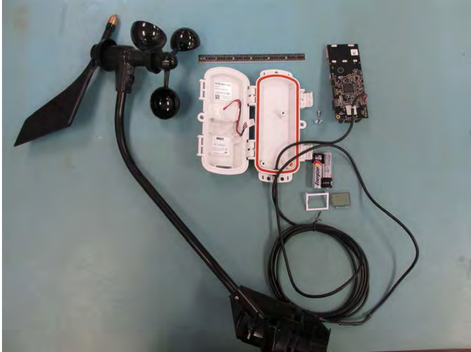
RXW-WCF-900 Exploded View with Sensor
