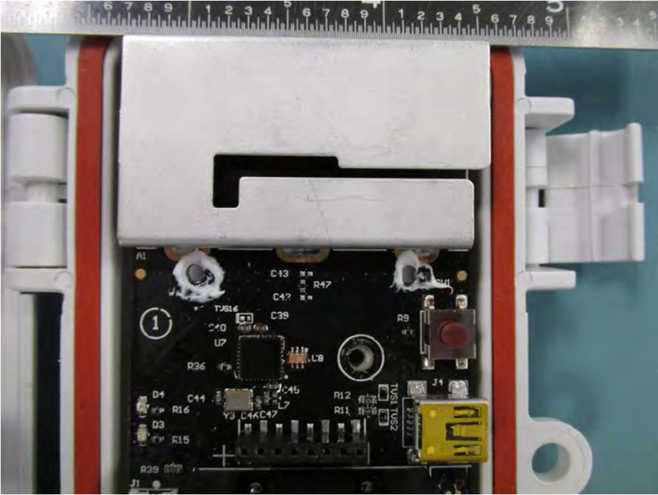
RXW-SMD-900 Radio Circuit
