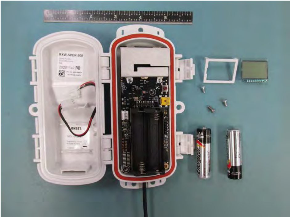
RXW-SPER-900 LCD Removed
