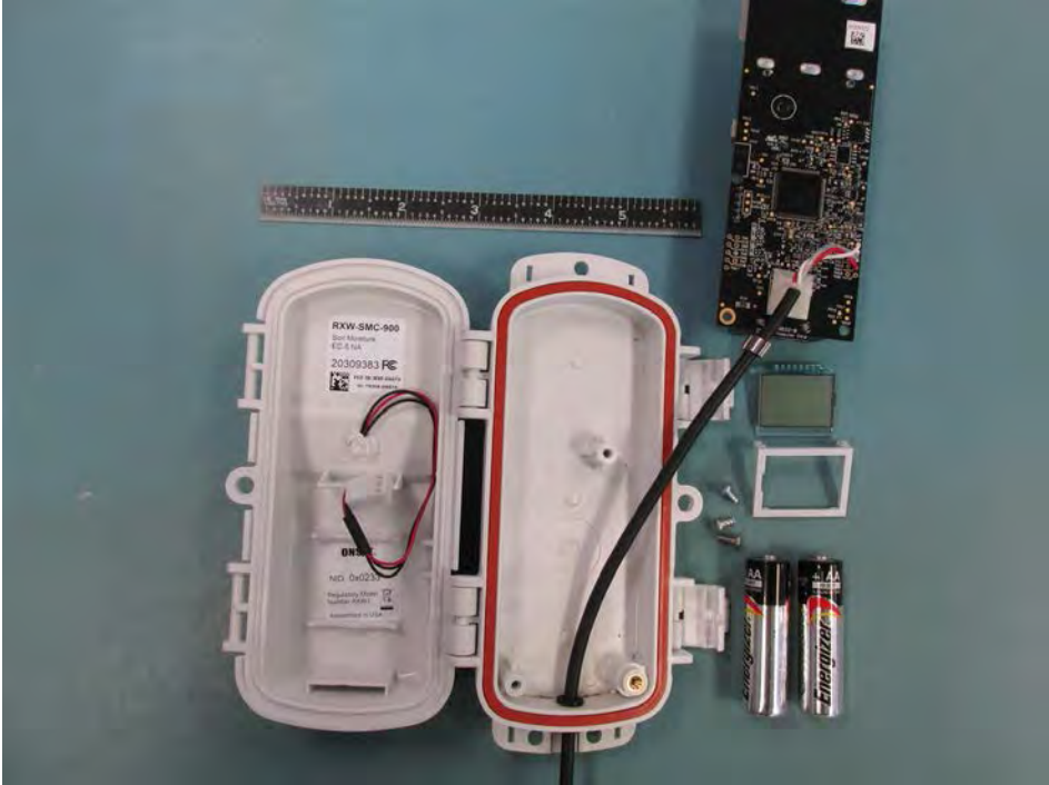
RXW-SMC-900 Exploded View
