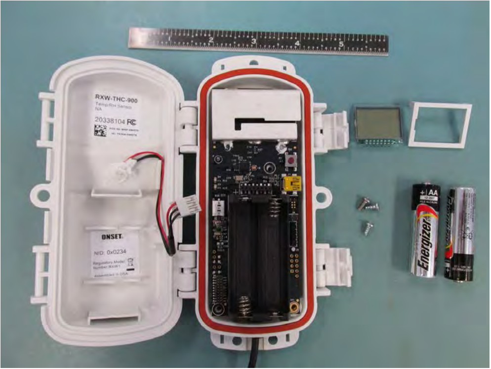
RXW-THC-900 LCD Removed
