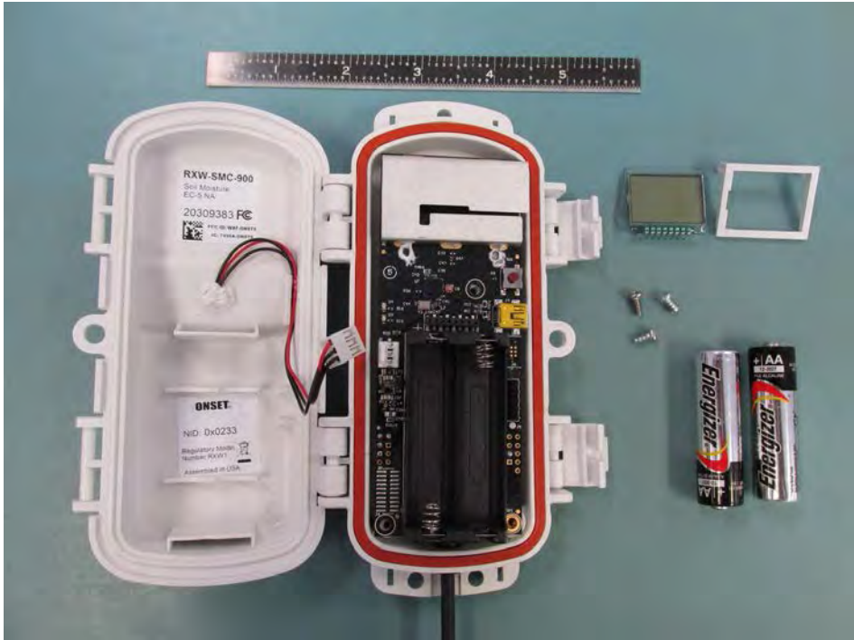
RXW-SMC-900 LCD Removed
