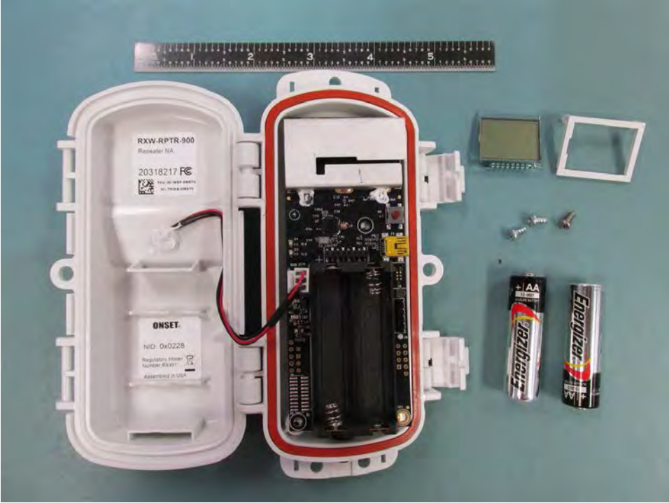
RXW-RPTR-900 LCD Removed
