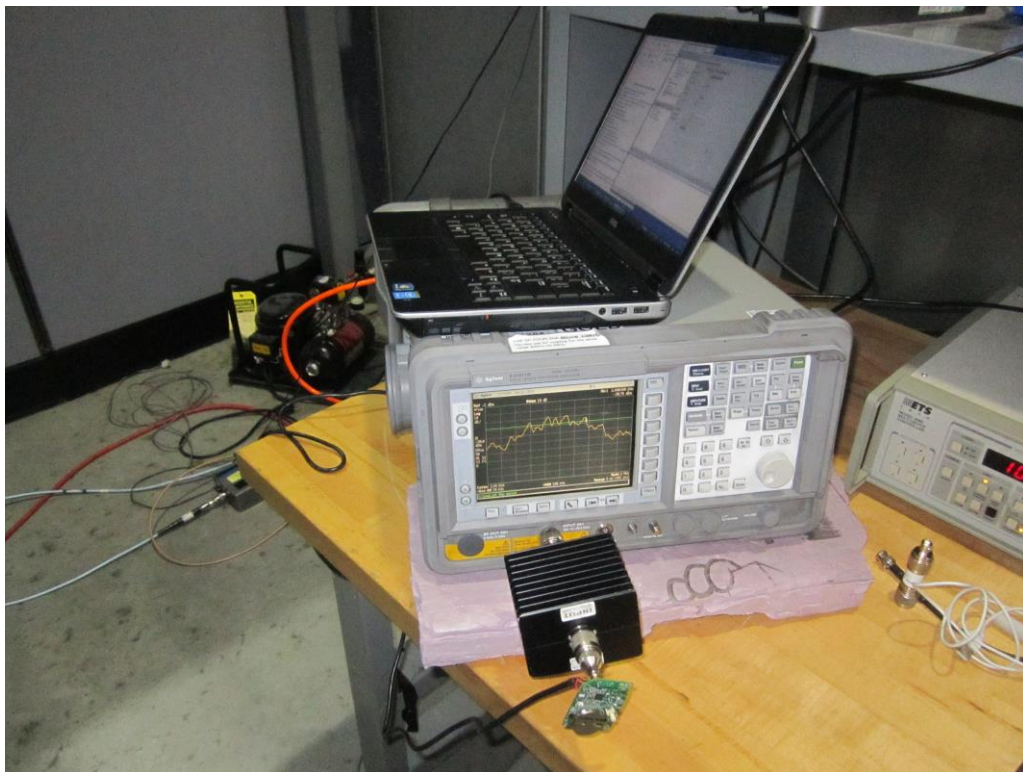
Conducted Emission at the Antenna Port (Setup Overview)
