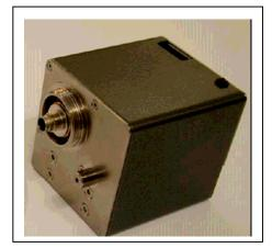
The DASY5 measurement server is based on a PC/104 CPU board with a 400MHz intel ULV Celeron, 128MB chipdisk and 128MB RAM. The necessary circuits for communication with the DAE electronics box, as well as the 16 bit AD converter system for optical detection and digital I/O interface are contained on the DASY5 I/O board, which is directly connected to the PC/104 bus of the CPU board.
