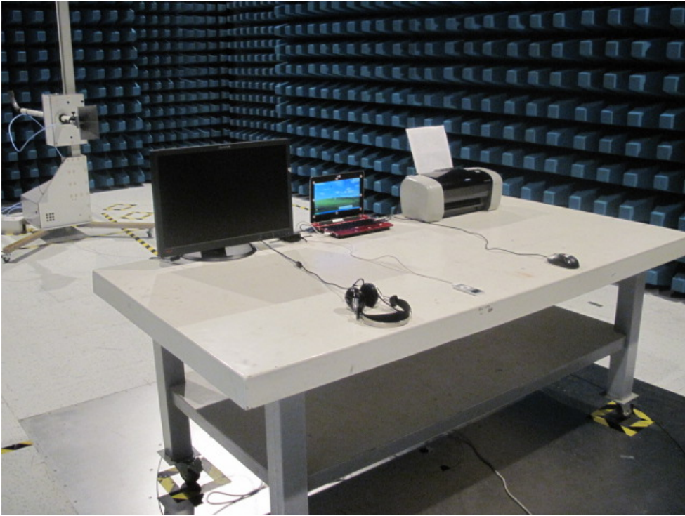
Description: Front View of Radiated Emission Test Setup for 1~18GHz
