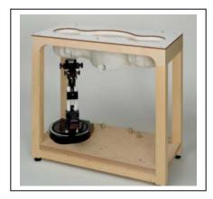
The bottom plate contains three pair of bolts for locking the device holder. The device holder positions are adjusted to the standard measurement positions in the three sections. A white cover is provided to tap the phantom during off-periods to prevent water evaporation and changes in the liquid parameters. On the phantom top, three reference markers are provided to identify the phantom position with respect to the robot.
