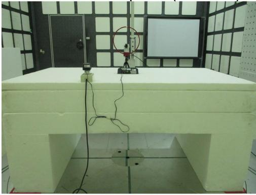
Radiated Emission Set up Photos (Below 1GHz)
