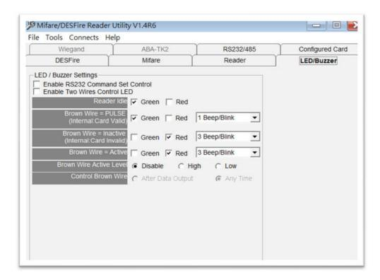
DF7XX supports LED/Alarm configure. Set the LED/Buzzer to indicate the system status for end-user.
