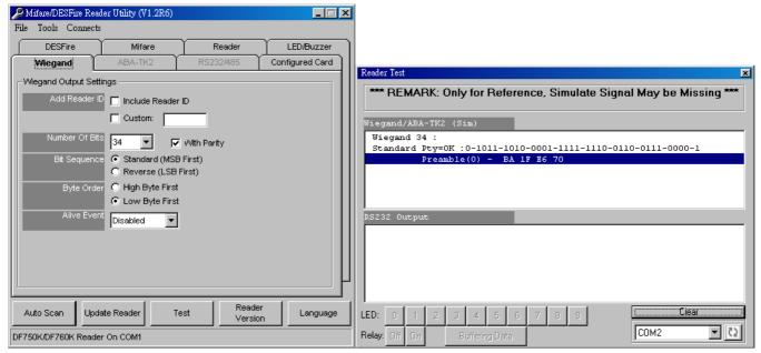
Remark: (1) When using reader-kit to test Wiegand (or TK2) signal, this test may be failed if the processor of computer is too slow. (2) When using reader-kit to test Wiegand (or TK2) signal, you need to connect to the physical COM port.
