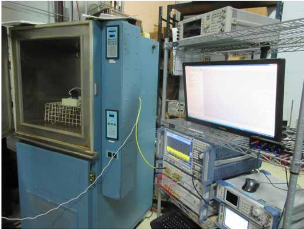
Test Setup for Antenna Conducted Emissions Tests
