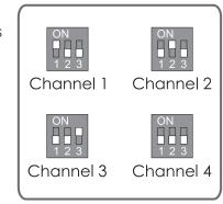
When refering to the diagram above, please take notice that the RF switch inside the battery compartment is located upsidedown.
