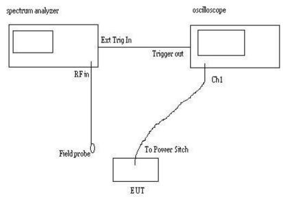
The spectrum analyzer was set in time domain, at 1 second sweep time, externally triggered. Connected to RF port is a field probe capable of capturing the RF signal of the EUT within close proximity.
