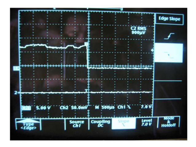
When the power switch of the EUT is released, the +5 to 0 V transition triggered the spectrum analyzer to initial a single sweep at sweep time of 1 second.
