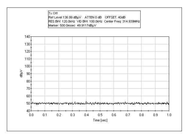
The above diagram shows instant cessation the transmit signal upon release of the switch, therefore comply with 15.231(a)(1) requirement.
