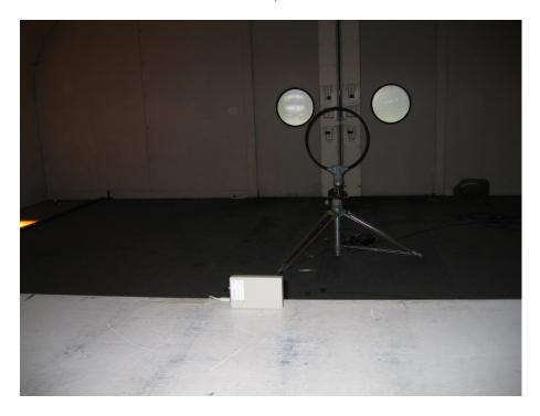
Radiated emissions, 30 MHz to 1000 MHz (front)
