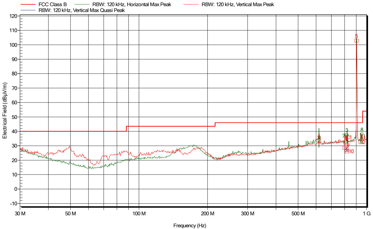
Figure 5.3.6.1: Electric field emissions Plot, 30MHz to 1GHz, ANT-868-CW-RAH Antenna - operation on Bottom Channel – Peak detector scan
