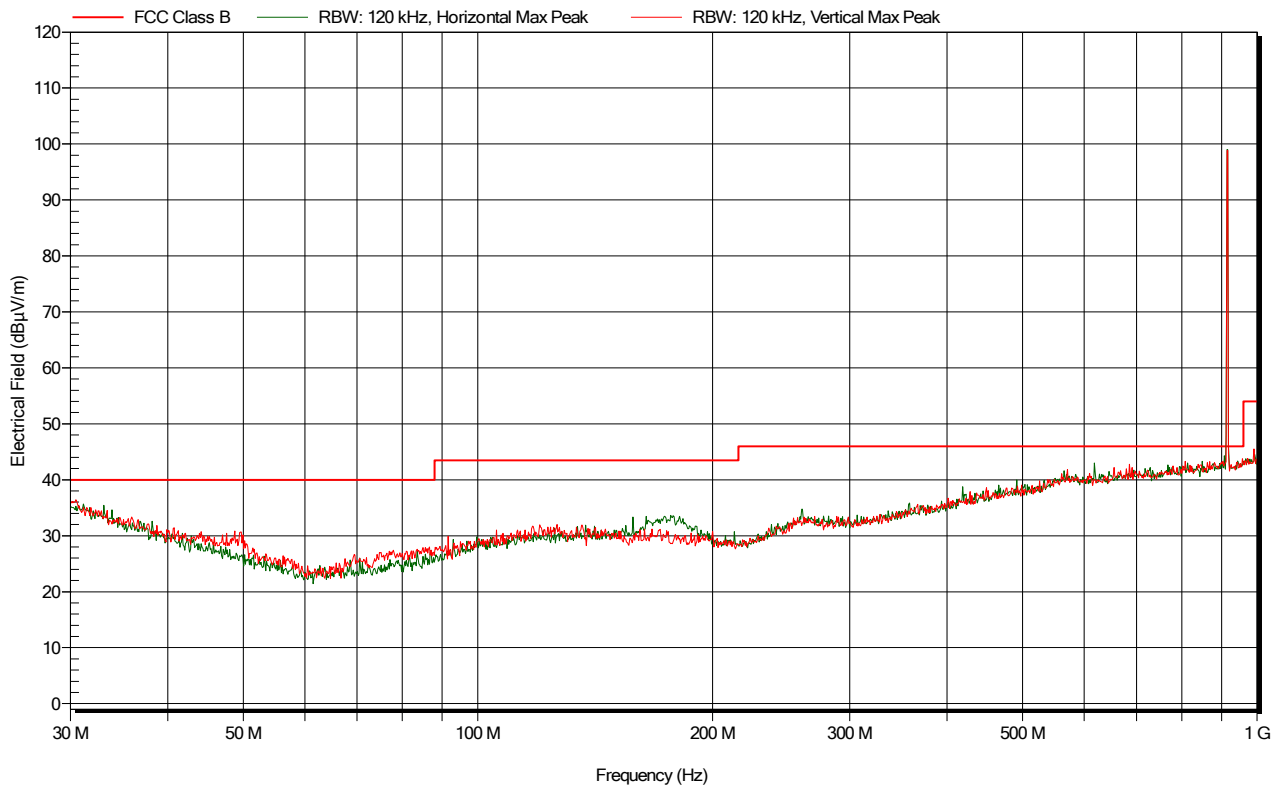
Figure 5.3.6.3: Electric field emissions Plot, 30MHz to 1GHz, ANT-868-CW-RAH Antenna - operation on Middle Channel - Peak detector scan
