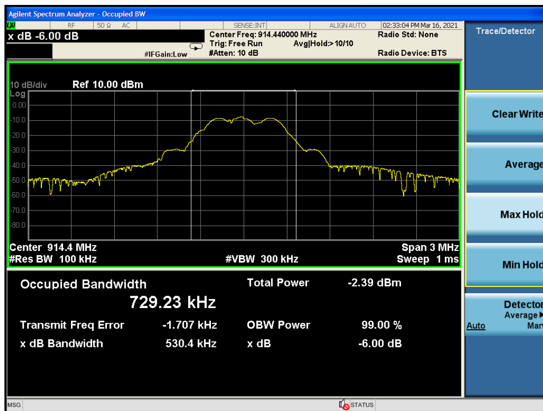
Figure 6.3.2 Bandwidth at 6dB Point. Operation on Middle Channel
