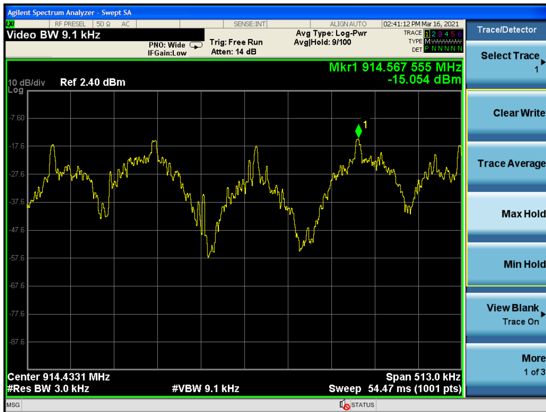
Figure 8.3.2 Power spectral density. Operation on Middle channel
