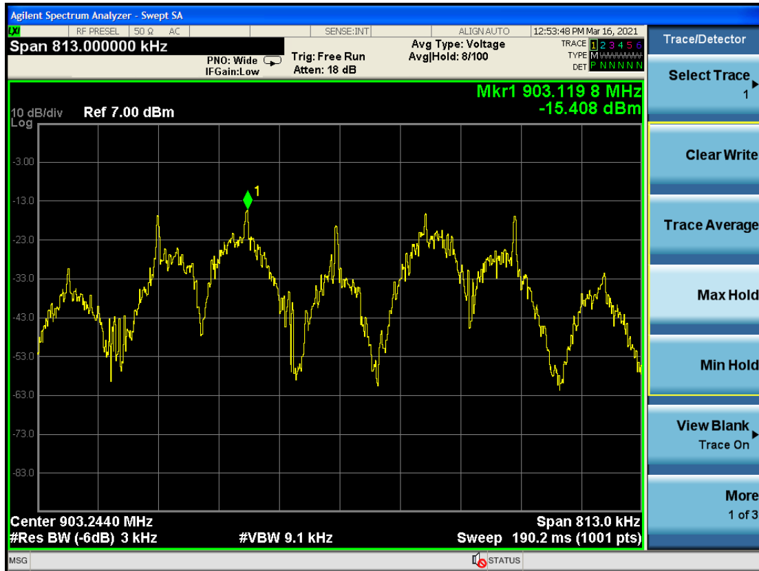
Figure 8.3.1 Power spectral density. Operation on Bottom channel
