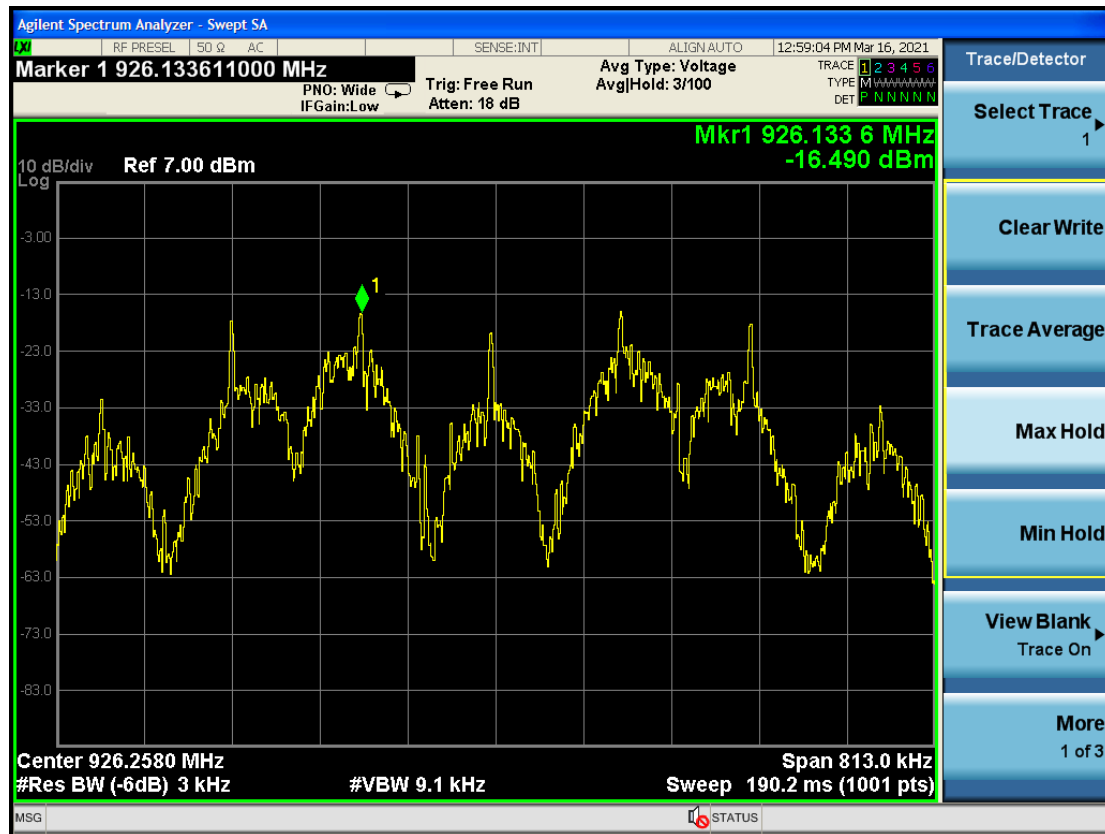
Figure 8.3.3 Power spectral density. Operation on Top channel
