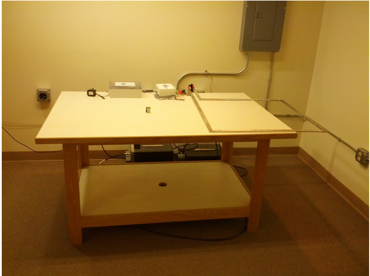
Front View Conducted Disturbance Worst Case Configuration
