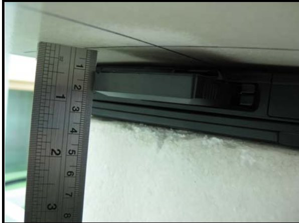
The bottom of the EUT face to the phantom with 10mm-separation distance.
