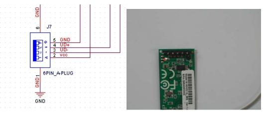
2. For using the module into your device, you should make sure the device has the same pin hole and the right pin definition. Below is the sample of wireless print server's main board. This print server has six pin holes and it is designed according to standard USB2.0. the pin hole's turn is from left to right.
