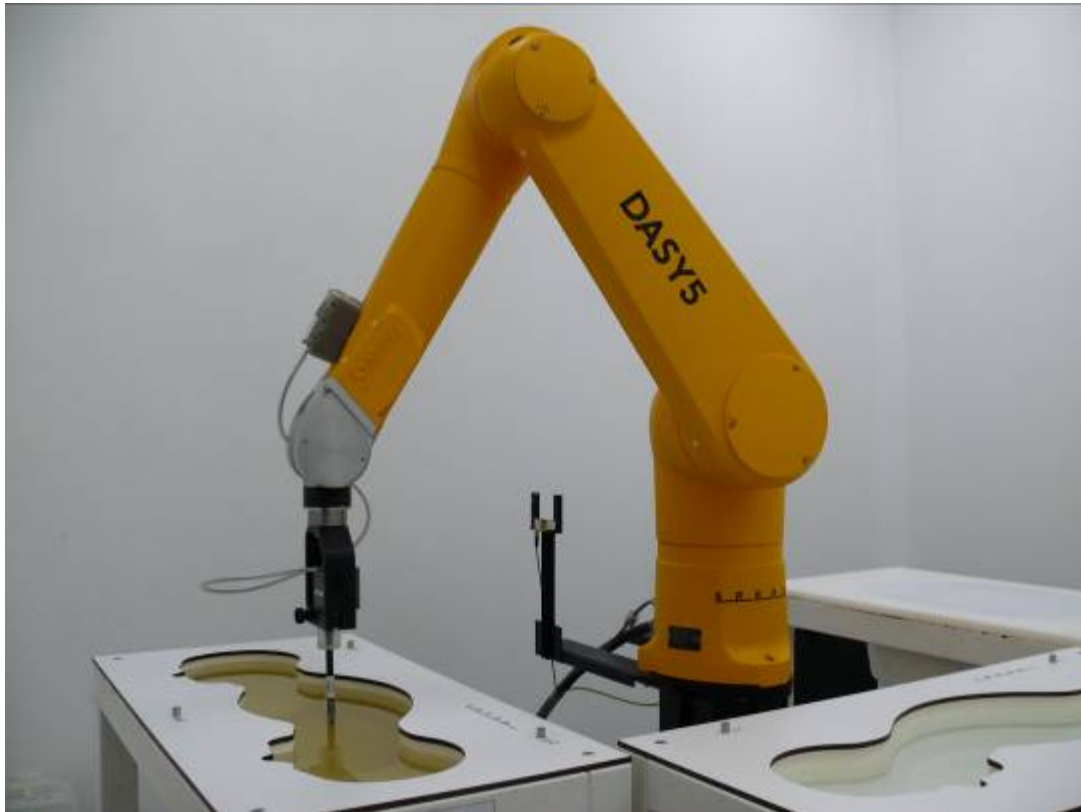
Picture 2: Specific Absorption Rate Test Layout
